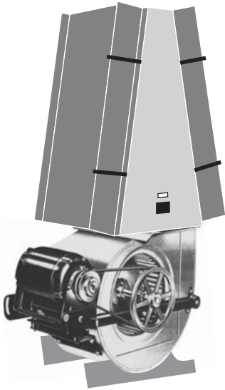
Figure 3-9 Typical open-frame industrial air purifier. Each filter unit contains one or more activated charcoal absorbers, including blower and motor. (Courtesy of Barneby Cheney Corporation.)
