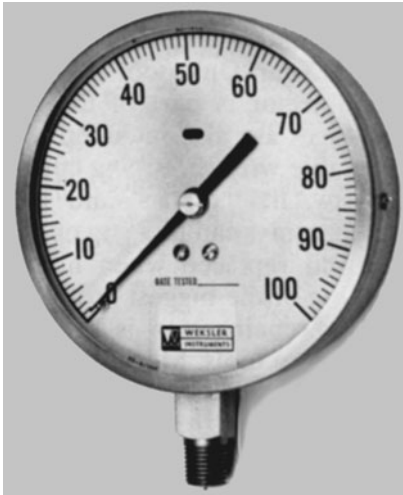
Figure 1-21 Pressure gage. (Weksler.)
