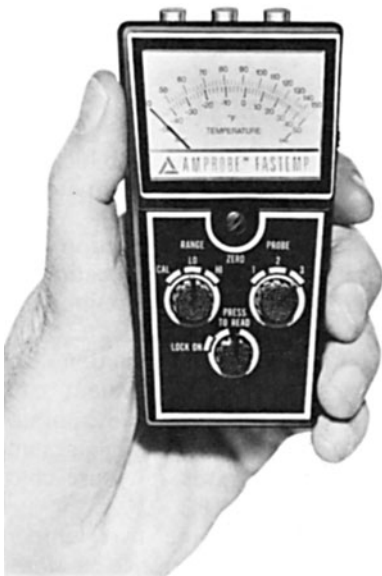
Figure 1-32 Handheld electronic thermometer. ( Amprobe. )
