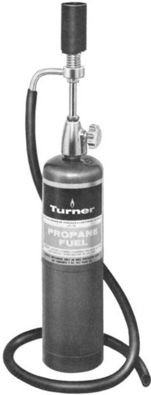
Figure 5-6 A halide gas leak detector. (Courtesy of Turner.)
