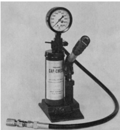
Figure 1-50 Cap-Check™ is a portable self-contained hydraulic power unit with auxiliary Equipment that is especially adapted to cleaning refrigeration capillary tubes. It is hand operated.
