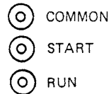
Figure 9-45 Built-up terminals on pancake compressors manufactured before 1952. (Courtesy of Tecumseh.)
