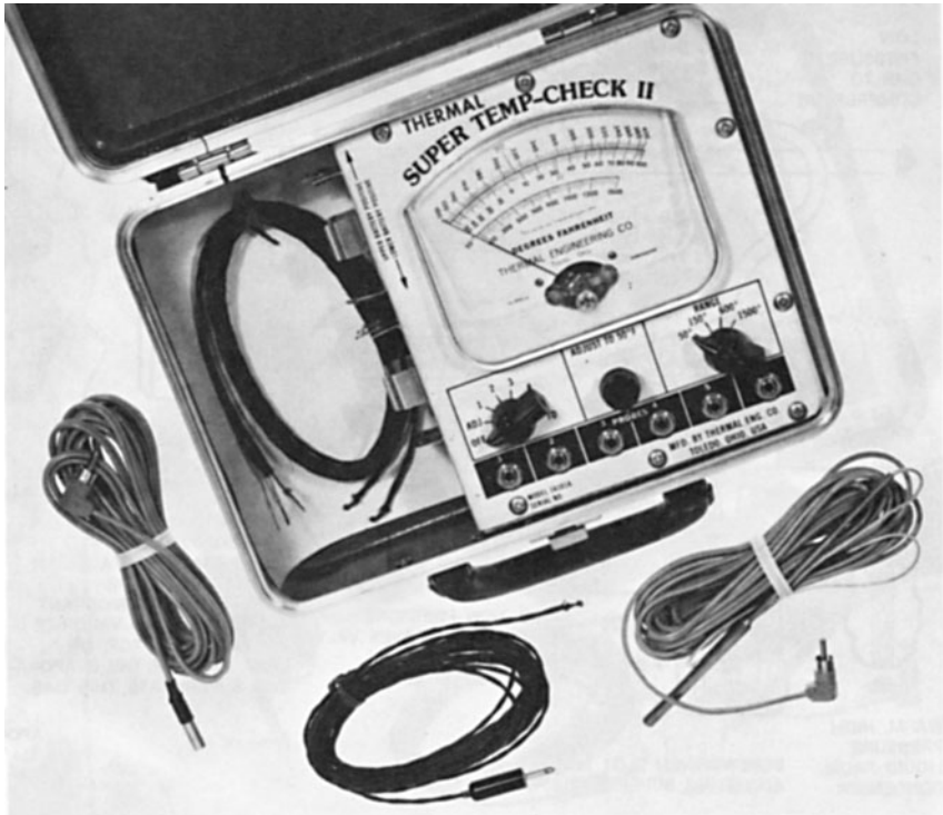
Figure 1-33 Electronic thermometer for measuring superheat. The probes are made of thermo-couple wire. They can be strapped on anywhere with total contact with the surface. This thermometer covers temperatures from -50^{\circ}\text{F} to 1500^{\circ}\text{F} on four scales. The temperature difference between any two points directly means it can read superheat directly. It is battery operated and has a \pm 2\% accuracy on all ranges. Celsius scales are available. ( Thermal Engineering .)
