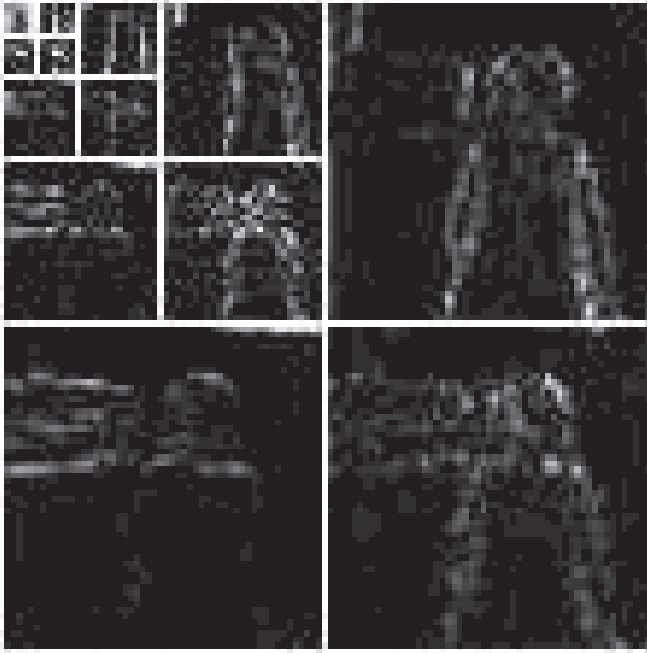
Fig. 3.30 The 2 dimensional discrete wavelet transform image coefficients arranged in a pyramid layout of depth four (see Figure 3.26).
