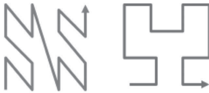
Fig. 6.28 Hilbert Space filling curve in 2 dimensions has less jumps then the Z -ordering.
