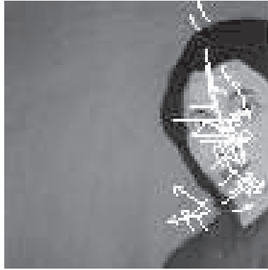
Fig. 5.12 Keypoints of the image of Figure 5.2. They are displayed as vectors indicating scale, orientation and location.
