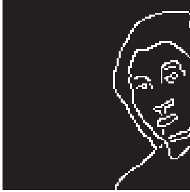
Fig. 5.4 Gradient image computed with the Sobel operator on the image represented in the Figure 5.2.
