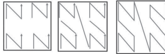
Fig. 6.24 The curve is generated recursively, four Z or N shapes are connected to form a order-2 Z-ordering.
