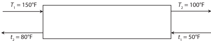
Figure 7.28 Ideal countercurrent heat exchanger; Example 7.5.
