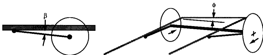
Fig. 6.16 Roll steer with a solid axle.
