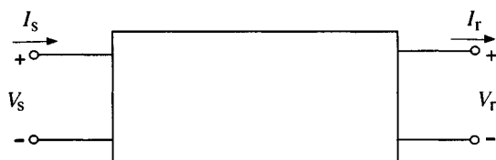
Fig. 8.9. Reference directions for current and voltage variables for ABCD parameters.
