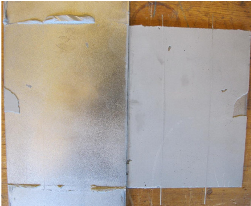
Figure 31.4: Connection 1 – side 1 – direction z+ (left side) and direction z- (right side) – third adhesive layer – complete delamination caused by adhesion failure
