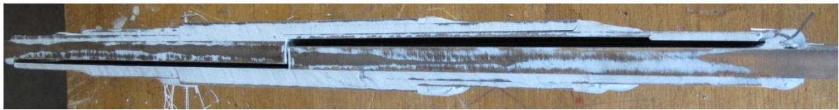
Figure 31.60: Connection 5 – Failure in Z-shape
