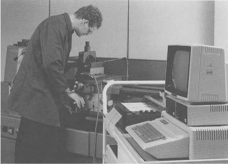
Fig. 2.18. Apparatus for testing cutting fluids to obtain quantitative data. [Courtesy of Cimcool.]
