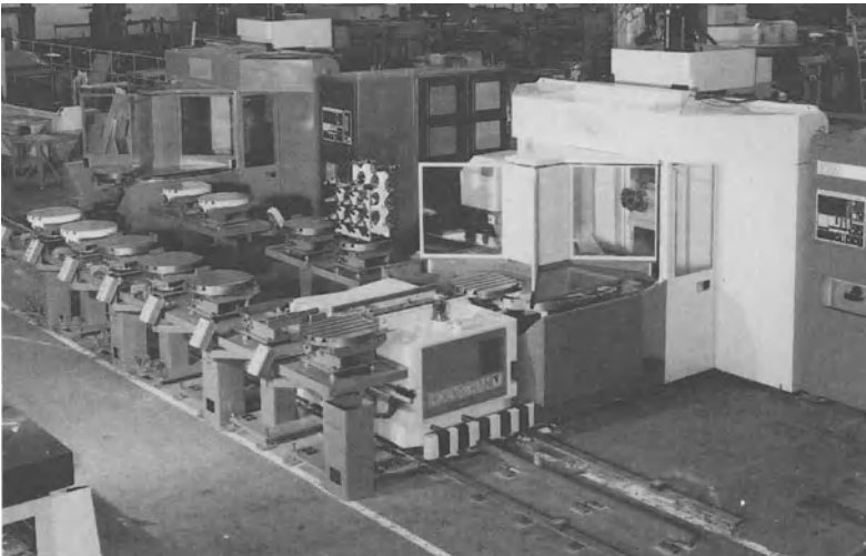
Fig. 3.28. A rail-guided vehicle (RGV) automatically delivering palletised workpieces and cutting tools to two horizontal machining centres in an FMC under test. [Courtesy of FMT.]
