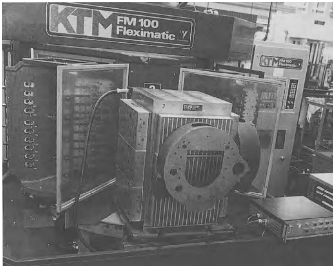
Fig. 3.24. A magnetic cube on a horizontal machining centre, with typical cutting data being: cutter diameter 160 mm (face mill); 268 r.p.m. (speed); 300 mm/min (feed); 4 mm (depth of cut); 125 mm (width of cut); 150 cm 3 /min (stock removal rate). [Courtesy of Eclipse Magnetics Ltd.]
