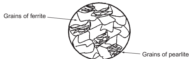
Figure 4.14 Microstructure of mild steel
