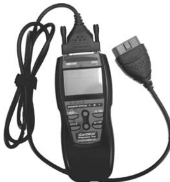
Figure 8.1 Picture of an OBD II scanner. [Source: picture taken in authors' lab]
