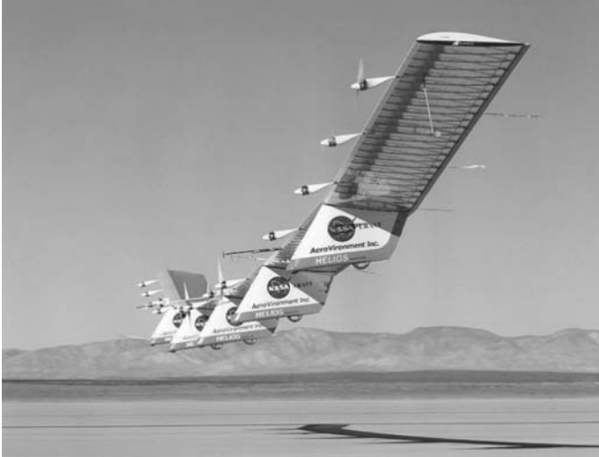
Figure 6.16 NASA's Helios Prototype solar aircraft. (Courtesy Wikimedia – original photo is from NASA.)
