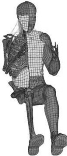
Fig. 13.69. THUMS (Total Human Model for Safety) developed by Toyota to improve the detail of responses obtained from virtual tests.
