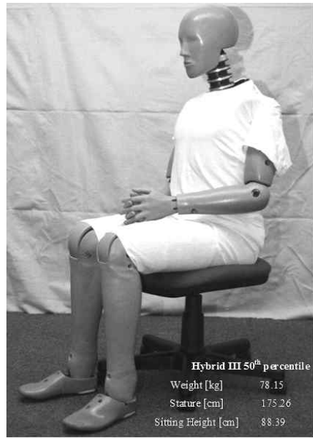
Fig. 13.64. Dummy for frontal impact: Hybrid III 50 percentile.
