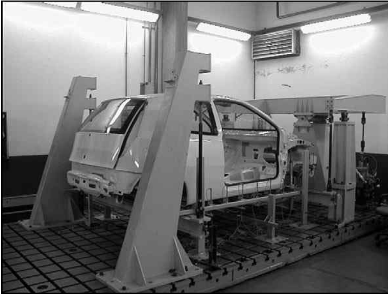
Fig. 12.68. Test bench for the measurement of the torsional stiffness.
