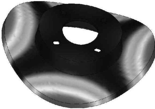
Fig. 11.38. Mode shape of a disk brake with two, orthogonal, nodal lines.
