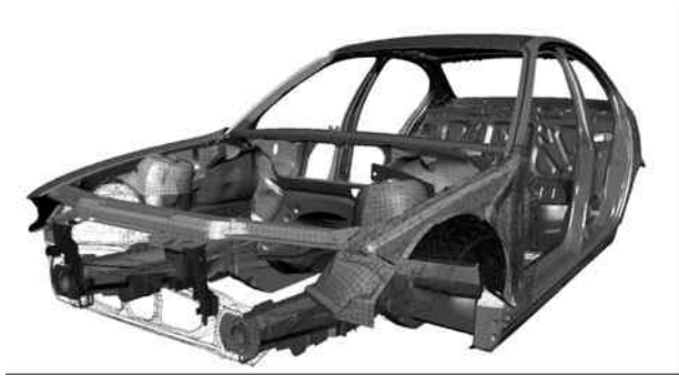
Fig. 12.64. Detailed FEM model of a car body structure. Most of the mesh is made by means of plate and shell elements.
