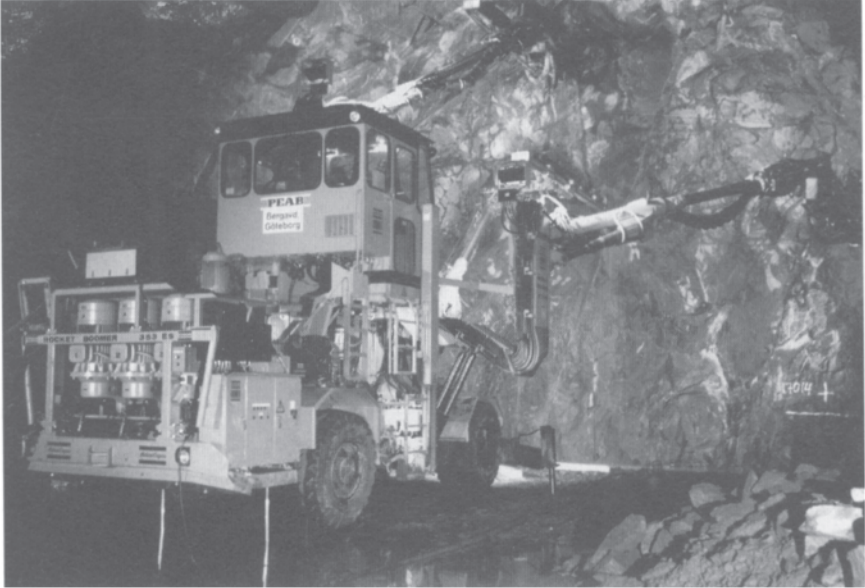
7. An Atlas Copco Rocket Boomer 353 ES drilling jumbo used for the Ullbro tunnel (photo by Shani Wallis).
