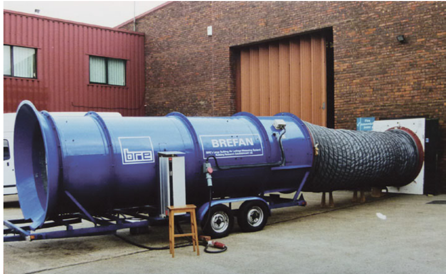
Figure 11.11 Testing for whole building airtightness
