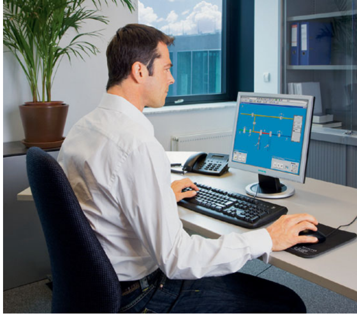
Figure 10.1 BEMS – A computer-based system (credit: Siemens)
