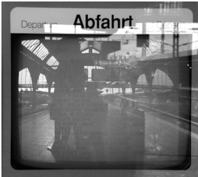
Figure 3-3. Reflected Glare on a computer display at a German rail station makes it impossible to read the arrival and departure information displayed, Photo credit: Panjasan (Own work) [CC-BY-SA-3.0 ( www.creativecommons.org/licenses/by-sa/3.0 )], via Wikimedia Commons
