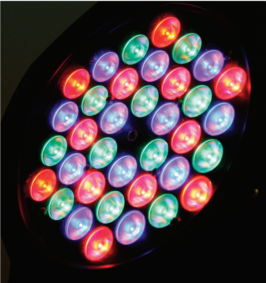
Figure A-4. A close-up of an RGB color mixing LED lighting fixture. By combining different colors, in this case Red, Green, and Blue, the primary colors of an additive color-mixing system, this fixture can create thousands of different colors and a variety of colored lighting effects.
