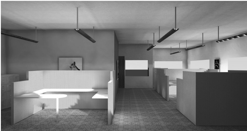
Figure 6-6. A 3D computer rendering generated by a radiosity calculation shows the interaction of light within an interior environment in a very naturalistic way. Image by AGI32 software.
