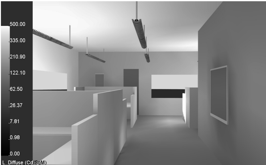
Figure 4-3. Luminance calculations displayed as a grey-scale gradient. Image by AGI32 software.
