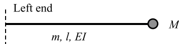
FIGURE 7.18. Design diagram of a beam; the left-hand end of the beam is free, or pinned or clamped.
