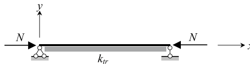
FIGURE 8.2. Beam on an elastic foundation.
