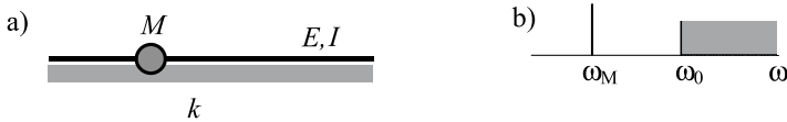
FIGURE 8.4. (a) Infinite beam with lumped mass on elastic foundation (b) Corresponding frequency spectrum.
