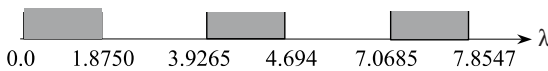
FIGURE 7.21(c). Clamped–free beam with a lumped mass along the span. Frequency spectrum.
