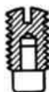
FIG. 171.—A variation of the preceding construction is obtained by making the plug a press fit in the screw.
