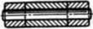
FIG. 119.—Common cover hinge with pin tight in the cover and loose in the hinge lugs.
