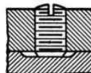
FIG. 169.—A flat filed or milled on the shaft is an improvement. But the cup point of the screw bites into the flat, and, once a ring is made into the flat, it is hard to get clear of it when the held member must be moved to either side.
