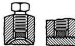
FIG. 173.—This is similar to the construction shown in Fig. 172, a tap being used instead of a reamer.
