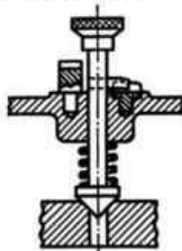
FIG. 71.—A long and a short slotted pin driven into the casting give two plunger positions.
