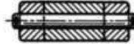
FIG. 121.—A plain pin with two cotters can be used in place of a peened rivet.
