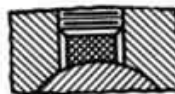
FIG. 172.—Here the side in contact with the shaft makes a full fit, achieved by inserting a reamer into the hub bore and constantly feeding the clamping screw while the reamer is turning.
