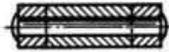
FIG. 120.—With the end peened, the pin can be made a loose fit in all lugs.
