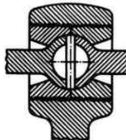
FIG. 158.—Socket joint with hemispherical rod ends held in place by screw bushings.
