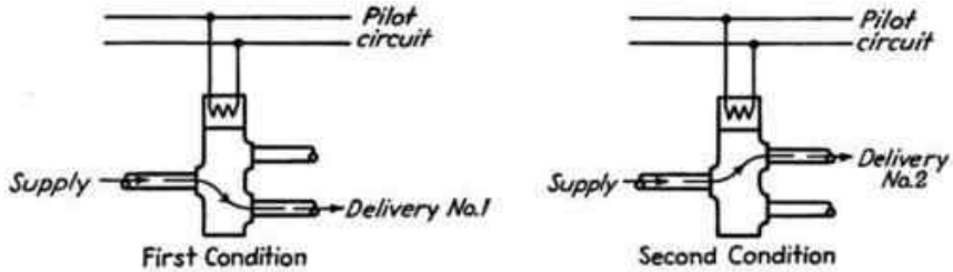
FIG. 473.—Three-way valve applied as convenient means of transferring one supply to either of two deliveries.
