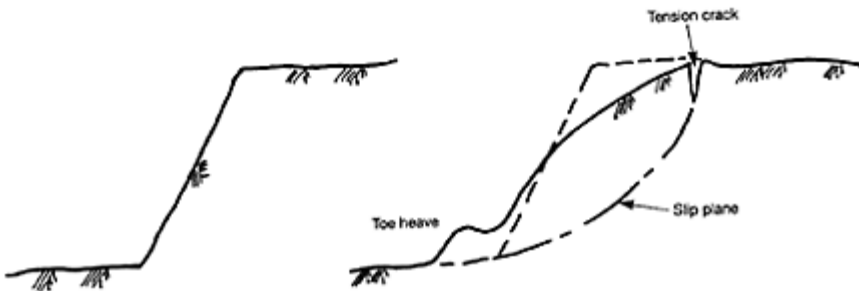
Fig. 7.1 Rotational slip: cohesive strata.
