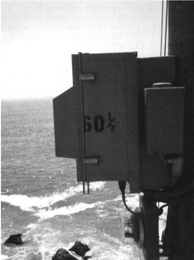
FIGURE 16.13 An optical converter (analog conversion) manufactured by Allen Telecomm.
