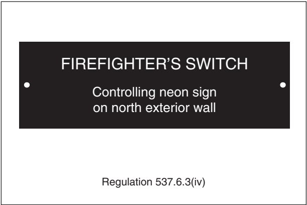
Figure 9.20 Remote fireman's switch notice
