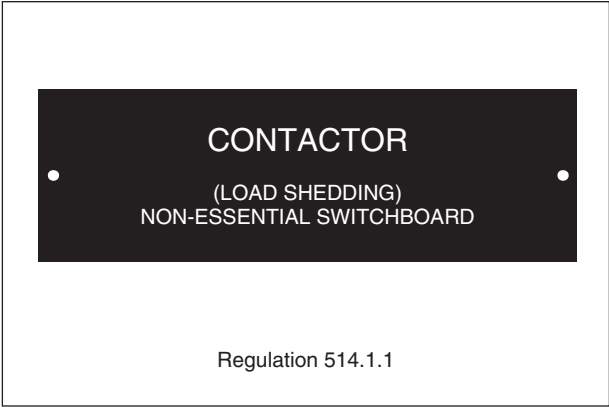
Figure 9.16 Contactor designation notice
