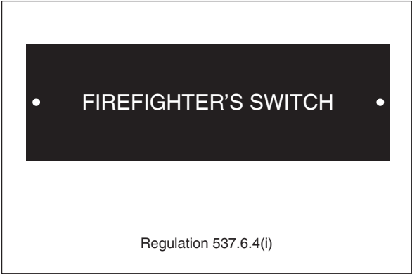
Figure 9.19 Firefighter's switch notice
