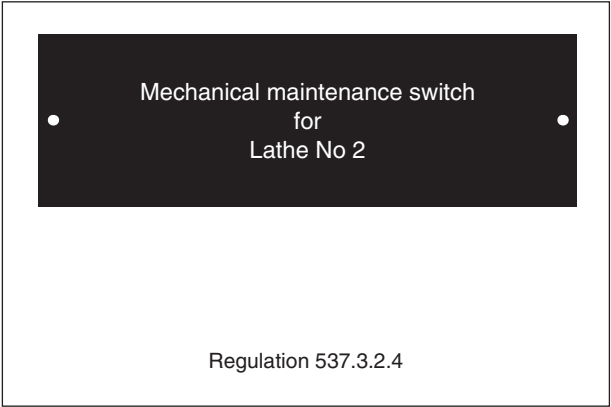
Figure 9.11 Mechanical switch notice
