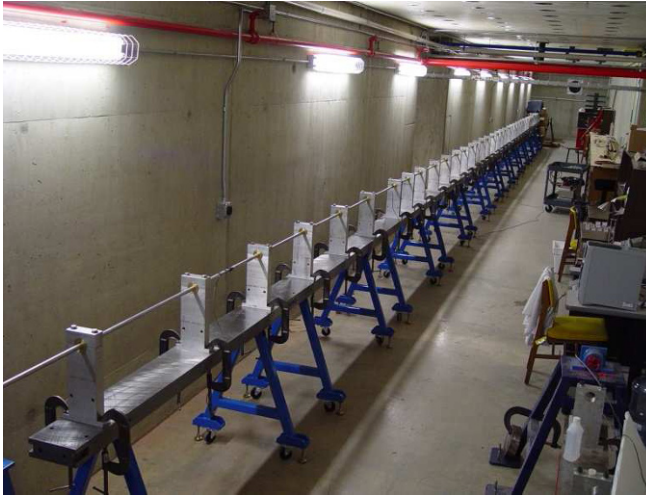
Figure 9.4 A photograph of a long Kolsky bar
