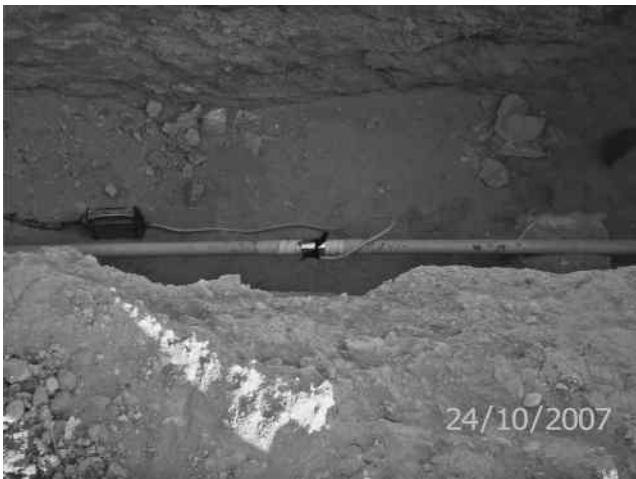
FIGURE 8.7 Radiographic test by gamma ray.
