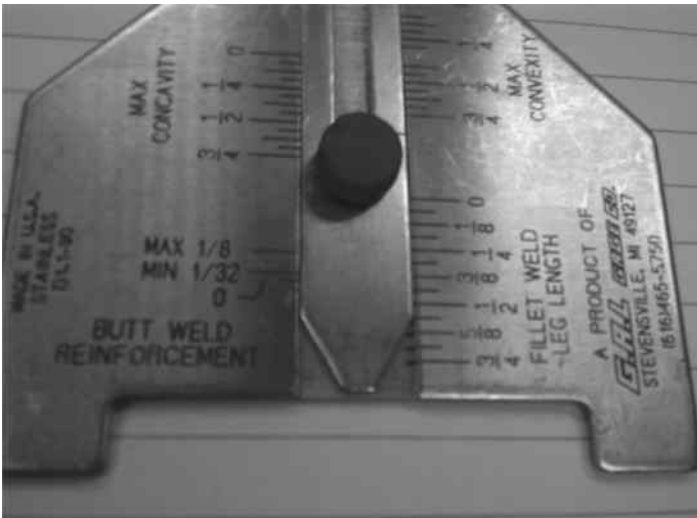
FIGURE 8.2 Butt weld thickness test.
