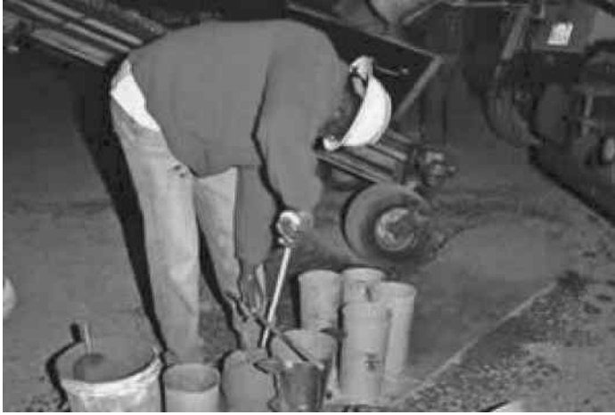
FIGURE 4.14 Measuring the slump settlement.
