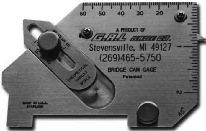
FIGURE 8.5 Multifunction tool for inspecting welding.
