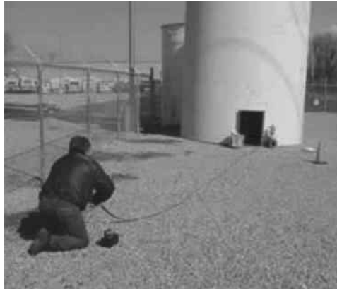
FIGURE 8.18 Maintaining distance between operator and source.
