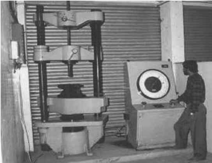
FIGURE 3.9 Steel bar in tension machine.
