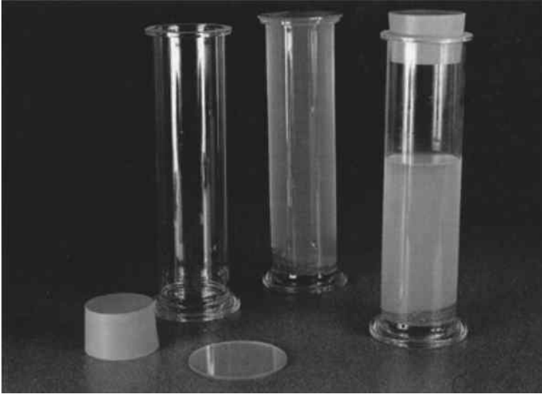
FIGURE 3.8 Tubes for aggregate density test.
