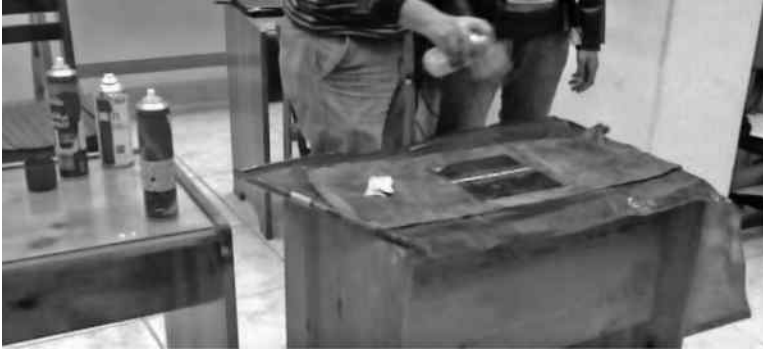
FIGURE 8.50 Using spray to develop, penetrate, and clean test surface.
