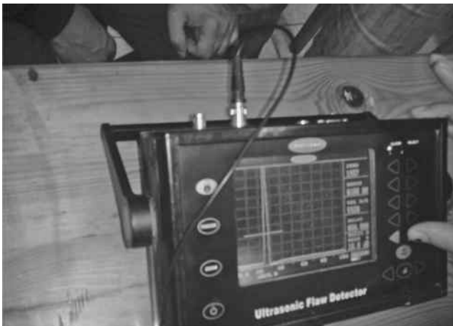
FIGURE 8.42 Echo pattern for discontinuity.
