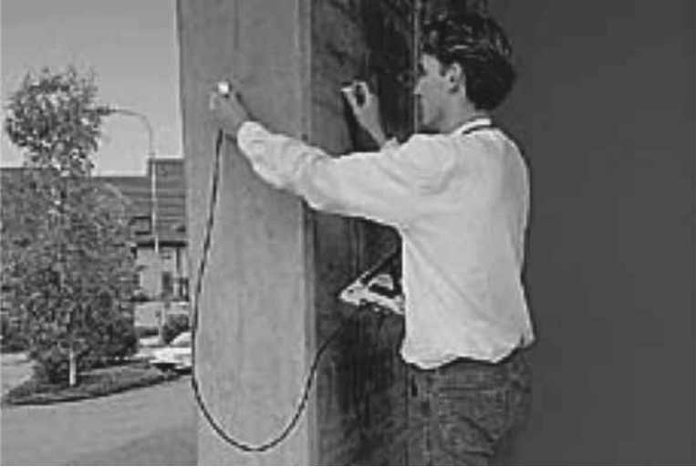
FIGURE 6.9 Semi direct transmission in progress.
