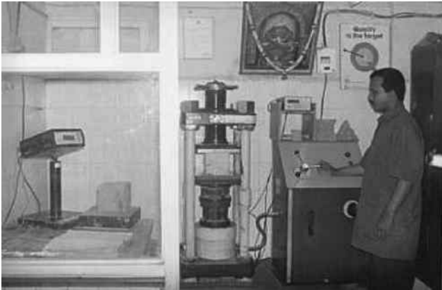
FIGURE 4.8 Compressive strength and density machine test.
