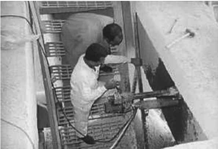
FIGURE 6.2 How to take a core.
