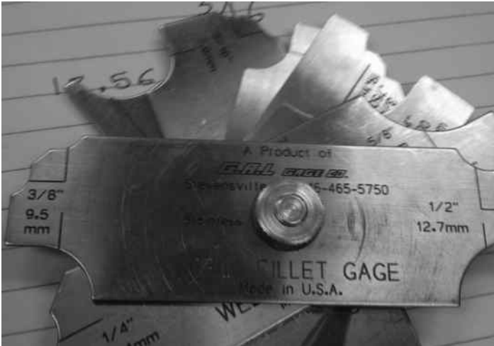
FIGURE 8.1 Fillet weld thickness test.
