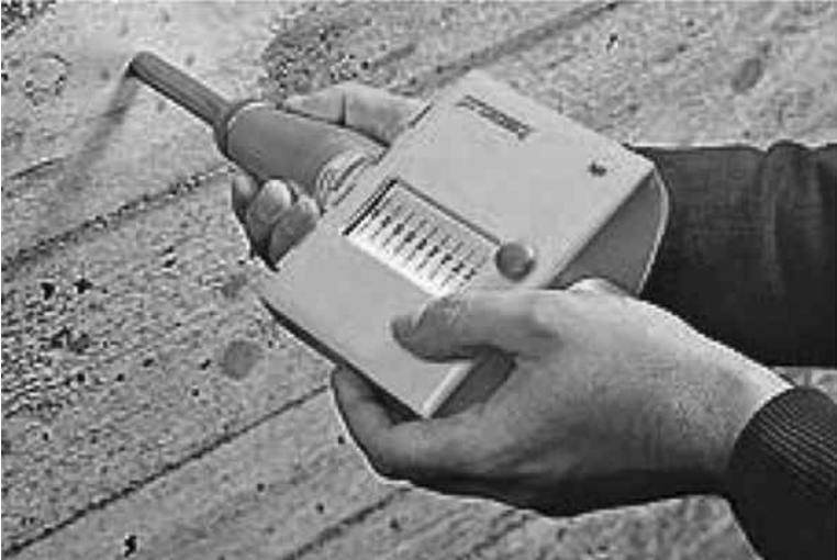
FIGURE 6.6 Rebound hammer test.
