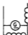
dc two wire generator (G) or motor (M), compound excited, short shunt
