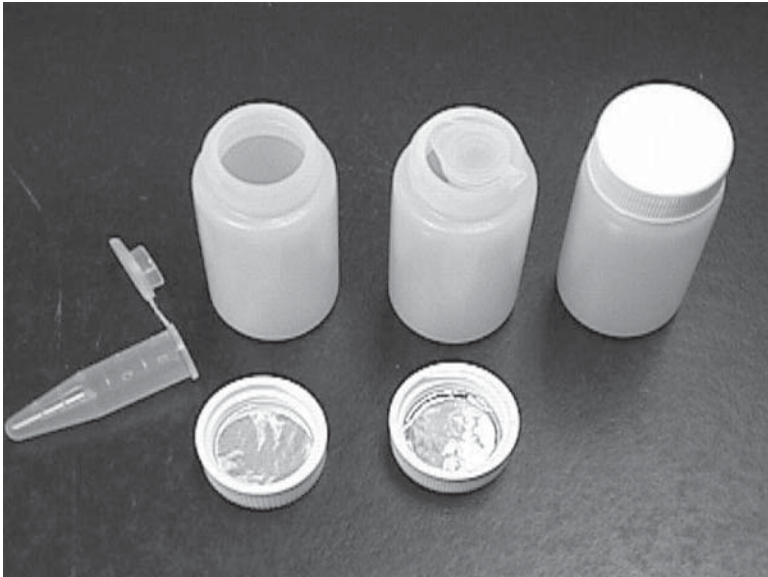
Fig. 7. Isolated radioactive beads and their competed supernatant fluids in separate Eppendorf tubes are individually placed into the tops of scintillation vials and capped for Cherenkov counting.
