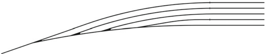
Fig. 8.29 Yard with curved tracks
