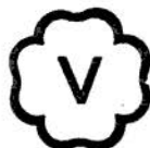
Fig. 5-9. ASME standard symbol for safety relief valves.
