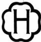
Fig. 5-8. Official symbol for stamps to denote ASME Standard Heating Boilers, Section IV.
