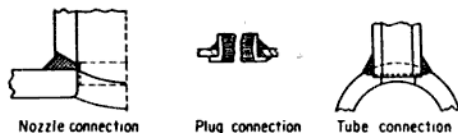
Fig. 7-6. Some types of welded nozzles and other connections to shells, drums, and headers, acceptable by the Code.
