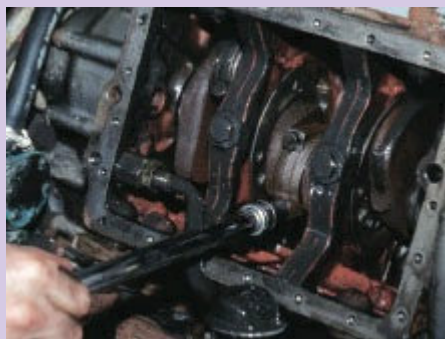
3 Loosen, then remove the big end cap nuts. To facilitate this, put the cylinder at bottom dead centre.
