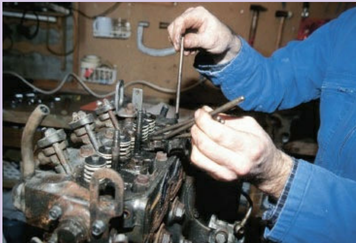
7 Remove the push rods one at a time.
