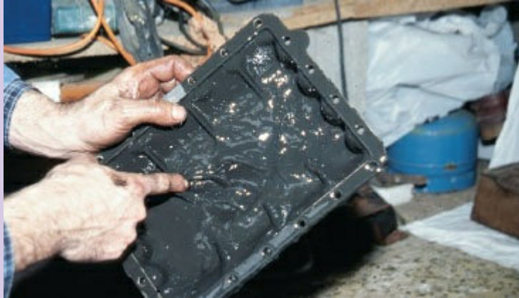
2 Note the deposits in the bottom of the sump.
