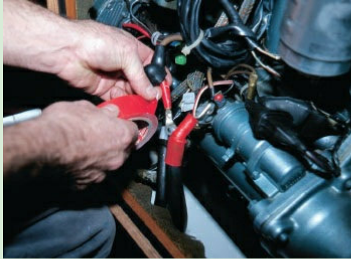
4 Electrical tape is an efficient way to mark them.
