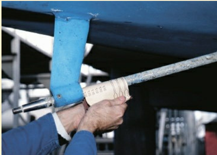
6 Before putting in the new bearing, it is important to clean the shaft lightly with sandpaper.
