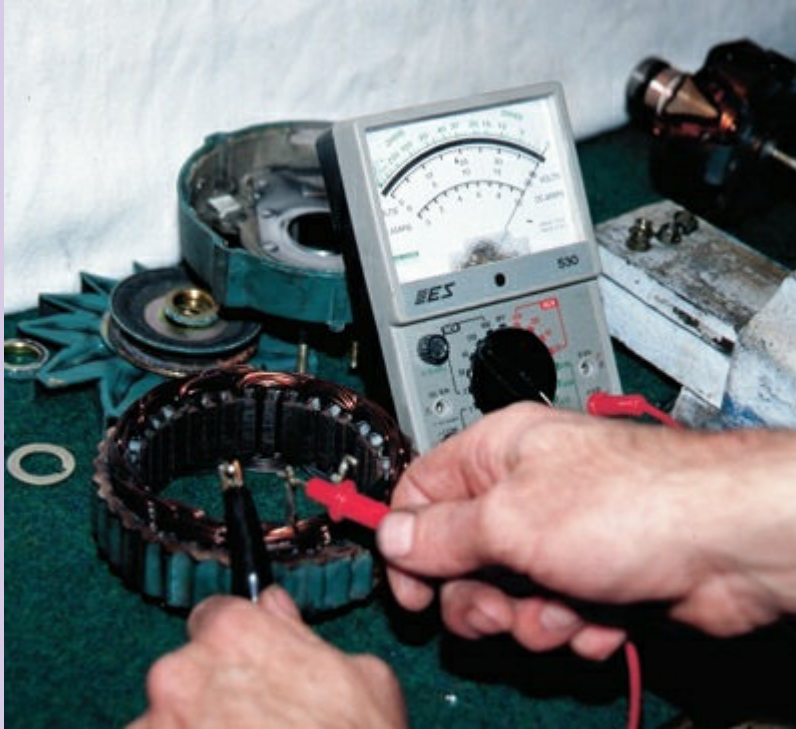
9 Testing the stator. Check each coil individually. The resistance should be the same for each coil (0.1 to 0.7 ohm). Check the insulation of the coils from the casing. (The resistance should read infinity.)
