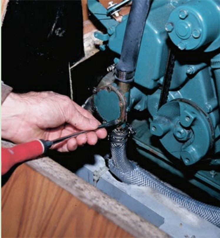
10 Put the cover plate with a new gasket back on the pump case.
