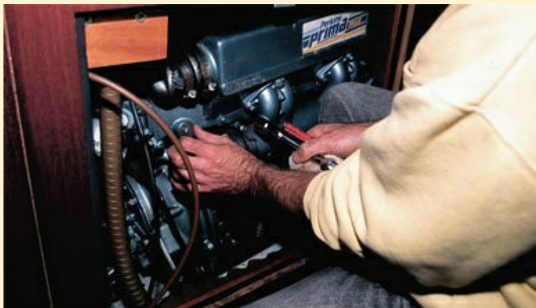
1 Locate the drain plug on the exchanger or the engine block.
