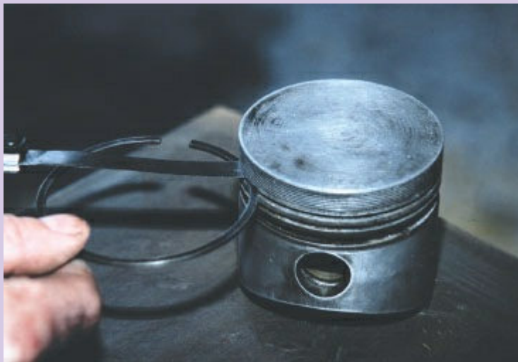
2 Carefully clean the pistons. Check the play of the rings in their grooves with a feeler gauge.
