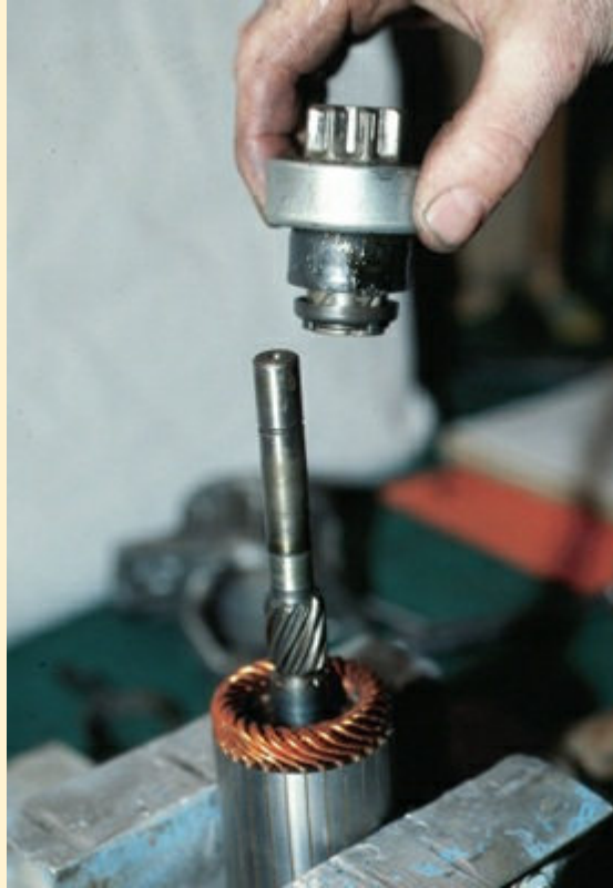
8 Remove the starter pinion from the armature shaft
