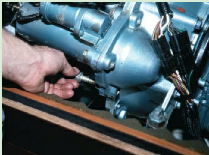
5 Now that all the wires are disconnected, you can remove the starter's mounting screws.
