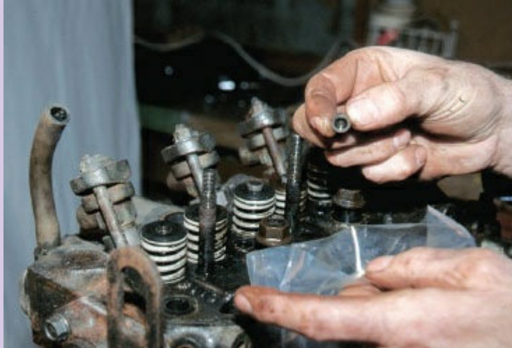
6 On Yanmar engines, remember to save the valve stem caps.
