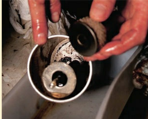
4 An accumulation of sediment! You should also always change the filter when you clean the bowl.
