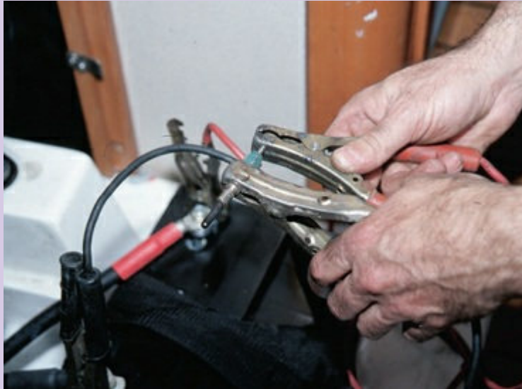
7 Feed the plug with about 10 volts of power with a battery jump cable. A lightly discharged battery connected in series can do the job.
