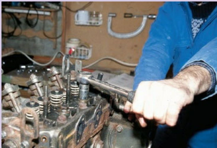
8 Loosen the head bolts, starting with the ones furthest away from the centre. These bolts
