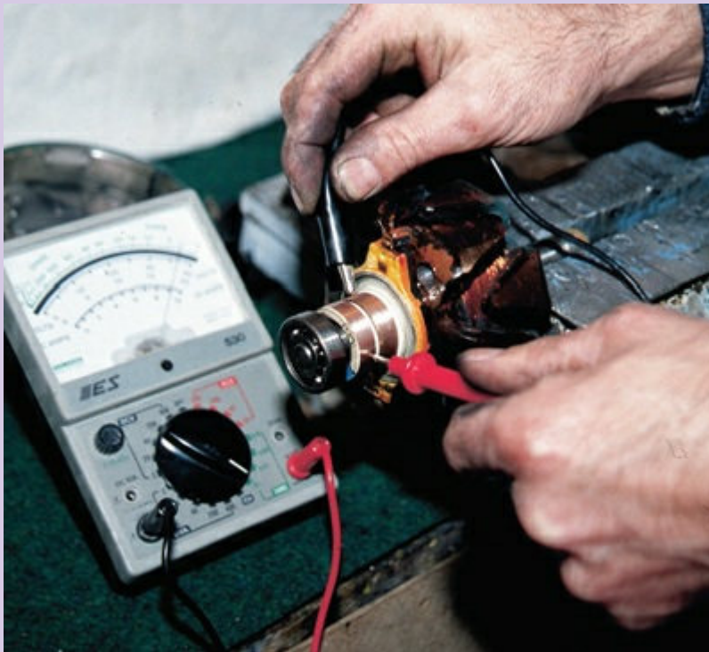
10 Test the rotor. Check the stator resistance (2 to 10 ohm) by placing the ohmmeter tips on each ferrule. Check the ferrule's insulation. (The resistance should read infinity.)
