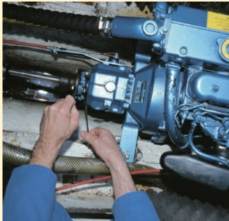
1 Unscrew and remove the nuts on the coupling.
