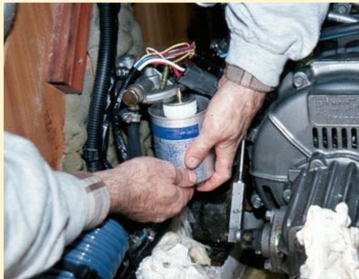
5 Clean the bowl. Remember to change the seal before reassembling.
