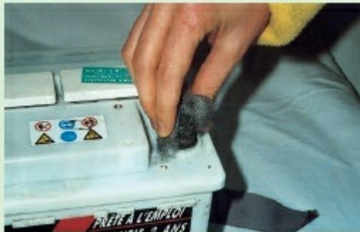
1 Clean the battery terminals.
