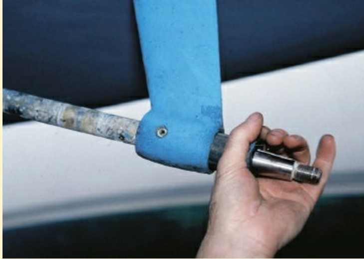
5 The worst is over; the bearing has been freed. You can remove it by hand.
