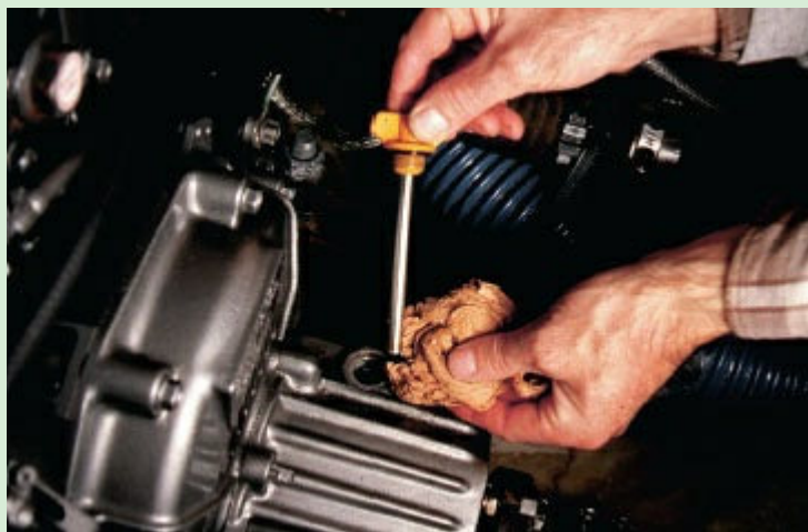
2 Wipe the dipstick clean, then re-insert it in the opening.
