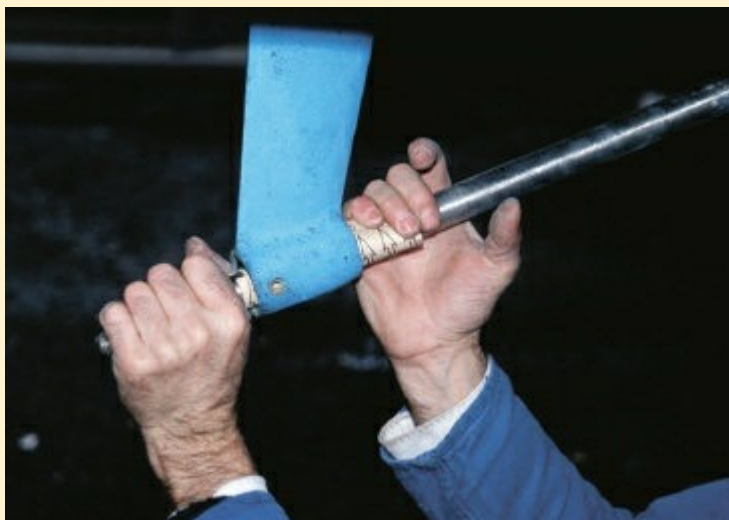
6 Before putting in the new bearing, it is important to clean the shaft lightly with sandpaper.
