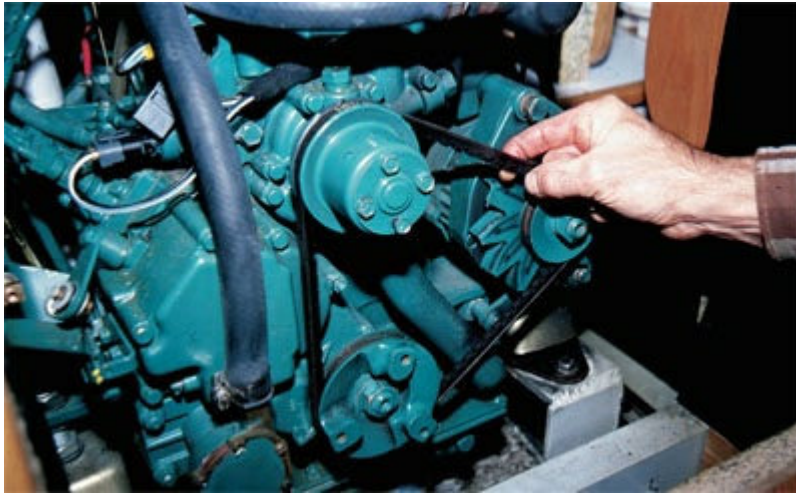
Checking the drive belt tension.
