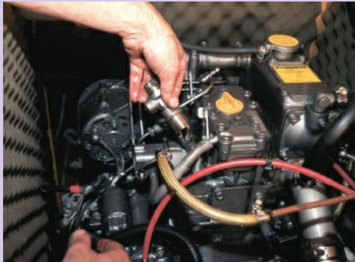
4 Move the high pressure line; remove the injector.
