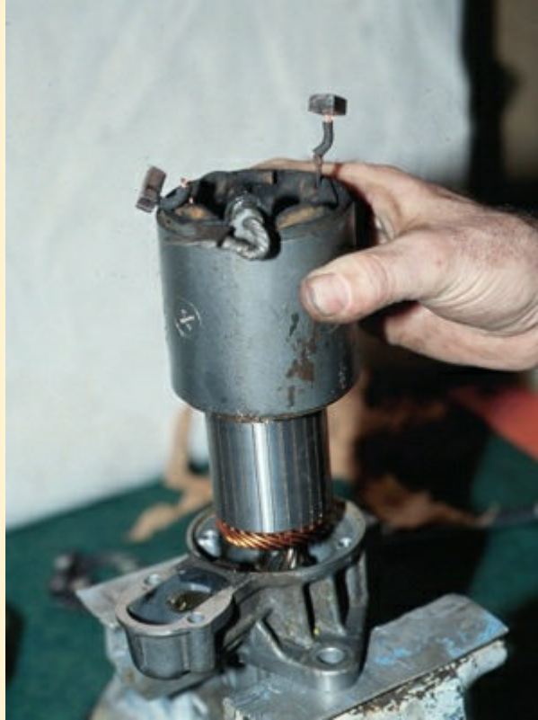
5 Remove the coil holder and the armature assembly.
