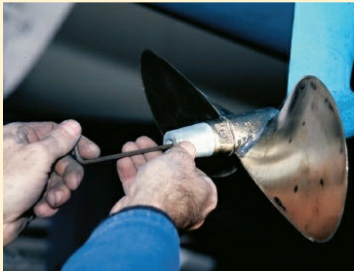
13 Screw a new anode on.
