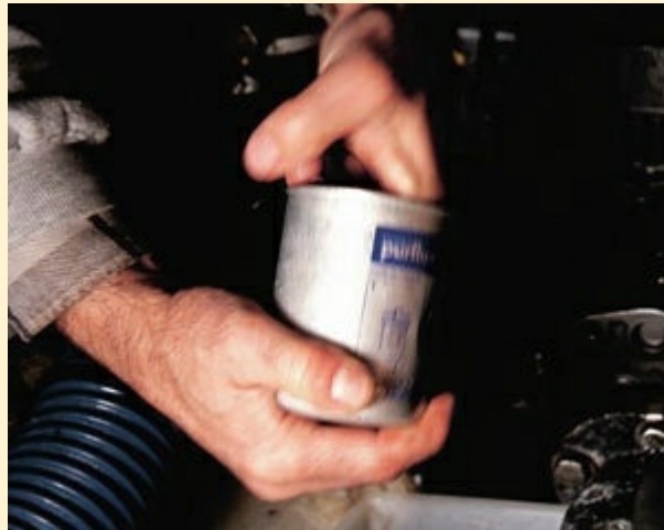
5 Clean the bowl. Remember to change the seal before reassembling.
