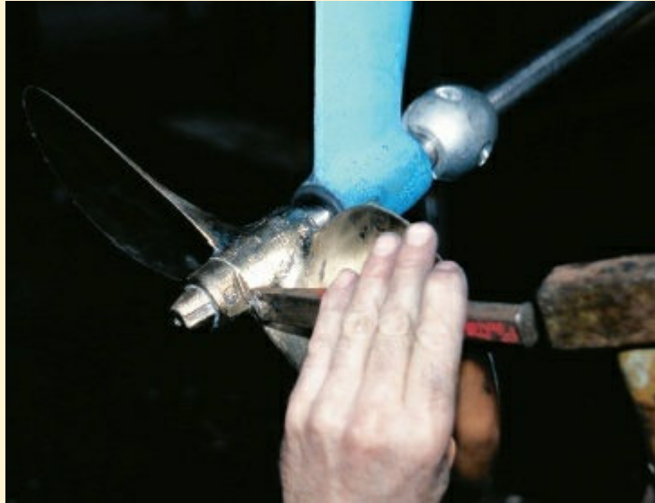
12 Fold over the lock washer tab.
