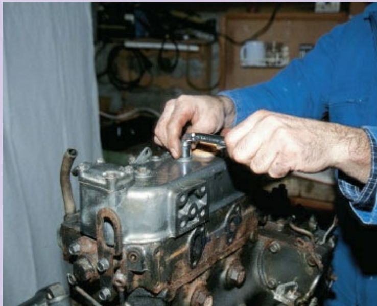
3 Remove the rocker cover. If it is stuck, use a wooden mallet.
