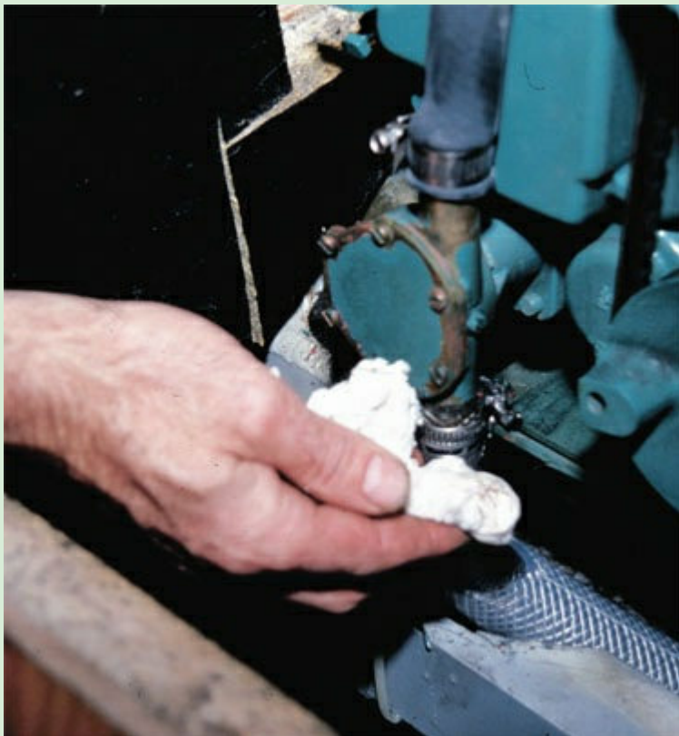
10 Put the cover plate with a new gasket back on the pump case.
