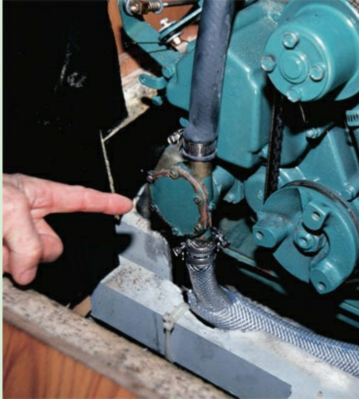
1 On most engines, the water pump is easily accessible.
