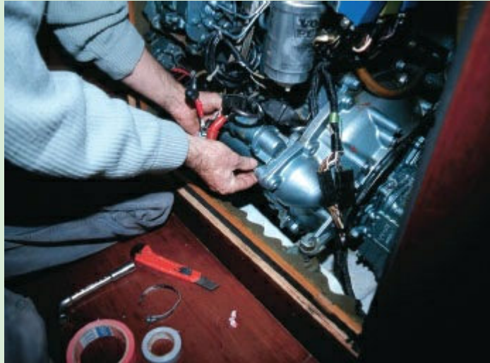
5 Now that all the wires are disconnected, you can remove the starter's mounting screws.
