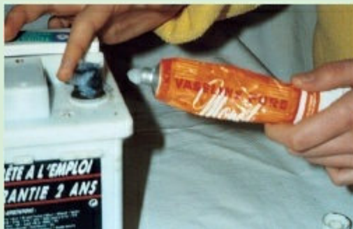
2 A little neutral grease (Vaseline) applied to the terminals inhibits the formation of salts.
