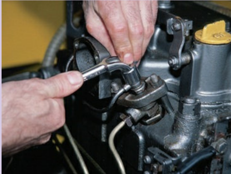
1 First loosen the leak vent-off pipe screw on the injector.
