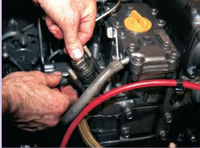
3 Loosen and remove the injector holding plate.
