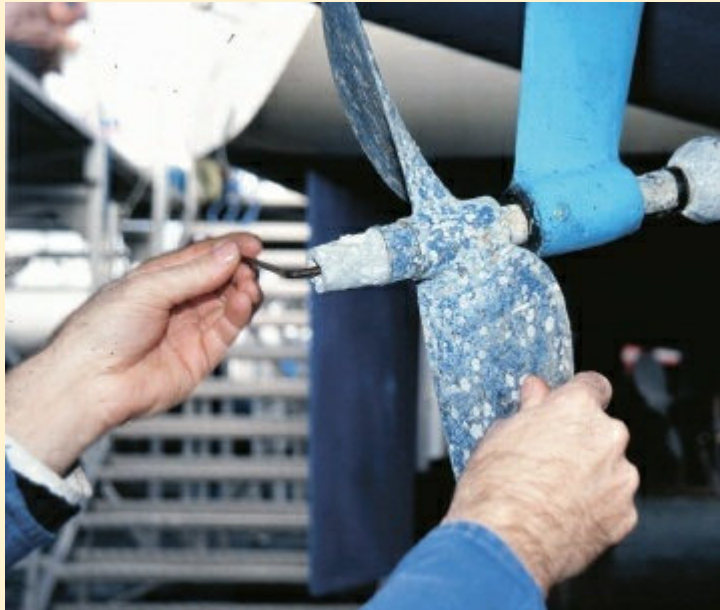
1 First, unscrew the anode with an Allen key.
