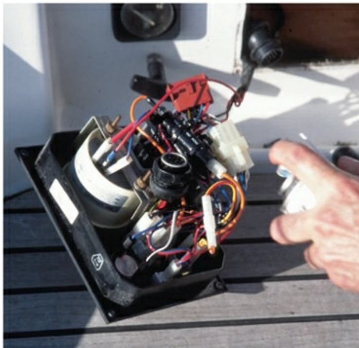
The connections and various components of the electrical circuit are very sensitive to
