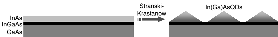
FIGURE 4.88 Schematic of Stranski–Krastanow epitaxy mode for self-assembled In(Ga)As QDs.
