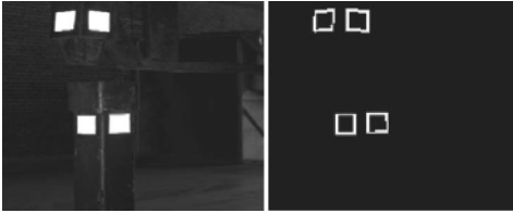
Figure 8.16 Retroreflective Fiducials. Here, squares of retroreflective tape are used to find the legs of parts racks that are to be aligned in order to stack the racks.
