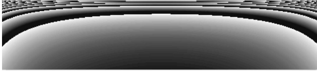
Figure 2.31 Image of Flat Terrain for the Azimuth Scanner. This image is for a height of 2.5 and a tilt of 16.5^\circ . Image intensity is proportional to range. To aid the visualization, wrap-around edges occur at equally spaced ranges.
