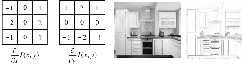
Figure 8.4 Sobel Operator. This is perhaps the simplest useful edge detector. The right image is the Sobel output for the kitchen scene. Each output pixel is an approximation of the gradient magnitude at the corresponding place in the input image. Vertical edges such as those in this image can be useful for localization.
