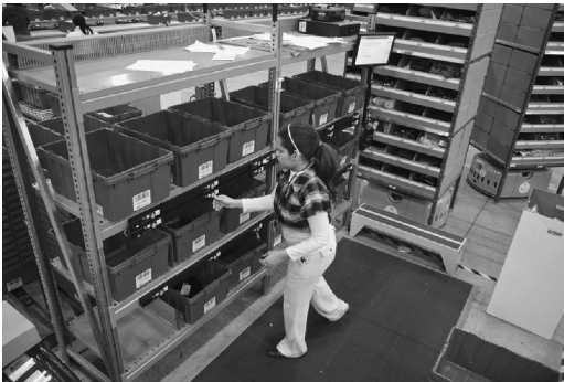
Figure 7.1 Kiva Systems Unit Load Robot. This robot is used to bring the racks in the distribution center to the order picking personnel. Feedforward terms in its controller turned out to be very important to its performance.
