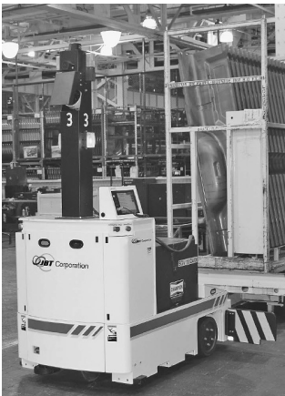
Figure 1.2 Tug AGV (JBT Corporation, Philadelphia, USA). These laser guided vehicles are used in factories to move materials from place to place.
