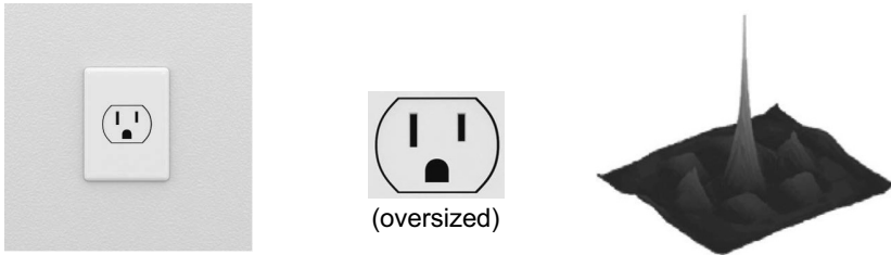
Figure 8.12 Template Correlation. If resources are available to compute correlation everywhere, it can be used to find the occurrence of the center image in the left one. The peak in the correlation signal occurs at the location of the closest match. As shown, the technique can be used by a robot to locate a plug in order to plug itself in to charge its batteries.
