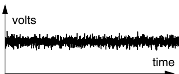
Figure 5.17 Bias of a Gyroscope Selection Random Process. Any randomly chosen gyroscope will have a noisy nonzero resting output.
