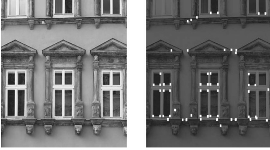
Figure 8.14 Harris Corner Detector. The Harris “corner” detector identifies features with high gradients in both directions. These are likely to be stable from image to image and hence, good candidates for matching and/or tracking.
