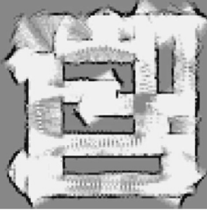
Figure 5.48 Results for Intuitive Model. Sharp corners are poorly defined but the overall map is recognizable.
