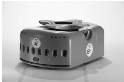
Figure 7.1 Kiva Systems Unit Load Robot. This robot is used to bring the racks in the distribution center to the order picking personnel. Feedforward terms in its controller turned out to be very important to its performance.
