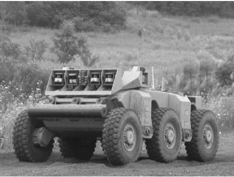
Figure 10.1 Crusher Robot. The Crusher robot was tested for several years on military bases throughout the United States. Its planner, based on the D* algorithm, regularly plans paths through natural terrain between waypoints separated by a few kilometers.
