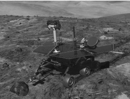
Figure 9.1 Mars Rovers. The twin Mars rovers Spirit and Opportunity have driven almost 30 kilometers across the Mars surface. As of this writing, Opportunity is still operating. Visual Odometry turned out to be a key technology for driving effectively in the fine Martian soil.
