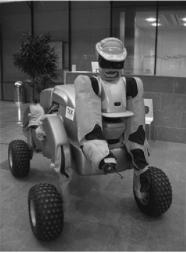
Figure 2.1 WorkPartner Robot. This robot is designed to not only get to the job, but it can do the job, too. The kinematic and dynamic modelling of this robot illustrates wheeled locomotion and dual-armed manipulation. To control this robot, models of both its mobility and its manipulation capability are needed.
