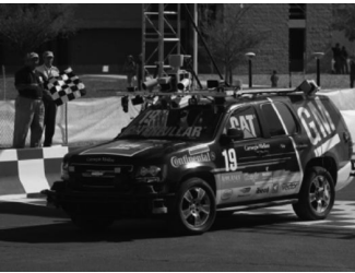
Figure 6.1 The “Boss” Autonomous Car. Boss is one of the six robots that finished the entire 2007 DARPA Urban Challenge course. The challenge was a test of driving in city streets with other robots and cars. Boss and most of its competition used very high performance inertial and satellite navigation systems.
