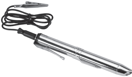
Fig. 18-28 A test light of this kind is convenient for tracing circuits, testing fuses, and so on.
