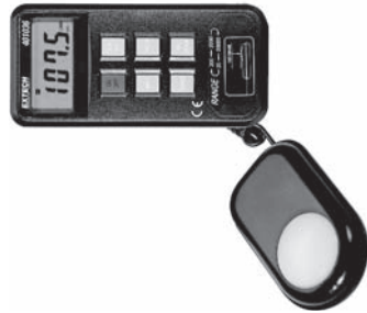
Fig. 14-3 The lightmeter indicates footcandles (or lux) of light directly on its scale. (Extech Instruments Corp.)
