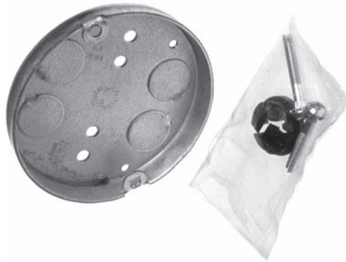
Fig. 21-1 This ceiling pan, with a volume of 6 cu in. and no required fill adjustments for an internal cable clamp, can just accommodate a single 14/2 AWG Type NM cable, or a 14, 12, or 10-2 AWG Type AC cable. (Hubbell Electrical Products)
