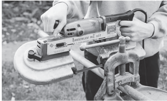
Fig. 11-4 If many cuts must be made, a power portable bandsaw is a good investment.
