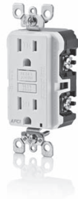
Fig. 6-11 This is an outlet branch-circuit (OBC) type AFCI receptacle capable of responding to both parallel and series failures on its load side, and series failures on its supply side. (Leviton)
