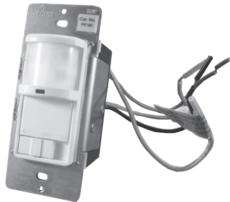
Fig. 5-33 An occupancy sensor type of switch, designed to replace conventional switches; the four leads are color coded, and allow for the switch to function as either a single-pole or three-way switch. The fourth lead is green and grounds the switch yoke as well as allowing the electronic controls in the switch to function with the lights off (see text).
