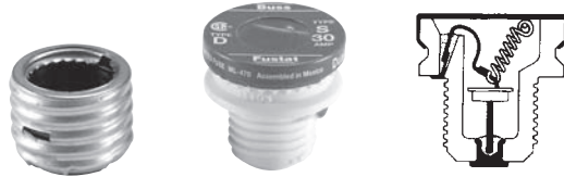
Fig. 6–3 A typical Type S nontamperable fuse (center and cross section at right) and its adapter. Once an adapter has been screwed into a fuseholder, it cannot be removed. This prevents the use of fuses larger than originally intended.
