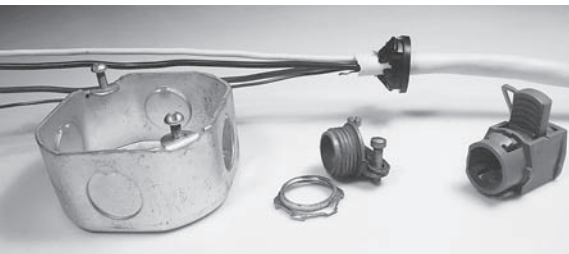
Fig. 11-28 An assortment of connectors for anchoring cable to outlet and switch boxes. The two-screw metal one near the center is also listed for two 12-2 or 14-2 Type NM cables.
