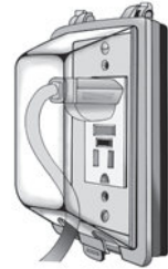
◀ Fig. 18–24 An outdoor receptacle in a weatherproof housing. It is suitable for damp locations and wet locations only while attended. ( Leviton Manufacturing Co. Inc. )
