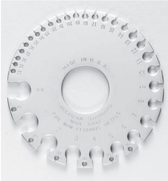
Fig. 7-2 A wire gauge shown slightly reduced in size. Measure the wire by the slot into which it fits. (General Tools Mfg. Co., LLC)
