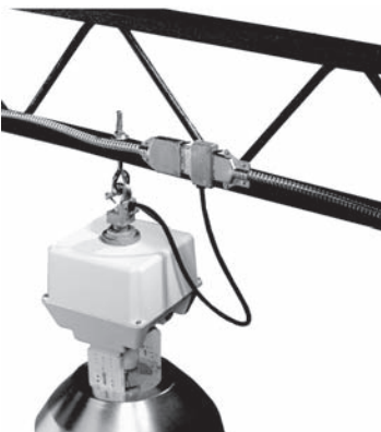
Fig. 31-2 A luminaire with a factory-installed receptacle for compatibility with a manufactured wiring system component. The system is energized through a plug designed to be connected to a specially configured receptacle mounted in a 4\frac{1}{16} -in.-sq box cover.
