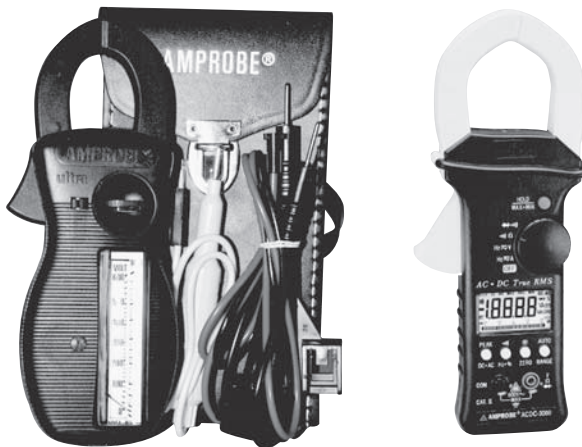
Fig. 2–2 Clip-on ammeters. They also have voltage scales. The one at the right can be used on ac circuits of widely differing frequencies, and even with dc circuits. ( Amprobe )
