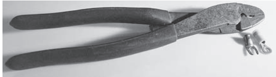
Fig. 8-18 This crimping tool has jaws for both insulated and uninsulated connectors.
