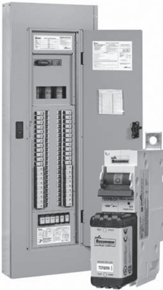
Fig. 28–1 A modern fuse cabinet supporting many branch circuits. The inset shows one of the branch-circuit modules, each of which contain an integral switch and a finger-safe removable cartridge that simplifies fuse replacements. ( Bussman Division of Eaton )
