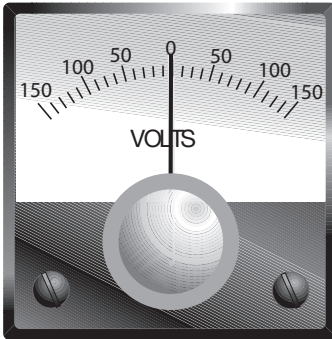
Fig. 3-1 This voltmeter is the same type as shown in Fig. 2-1 except that the zero is in the center of the scale.
