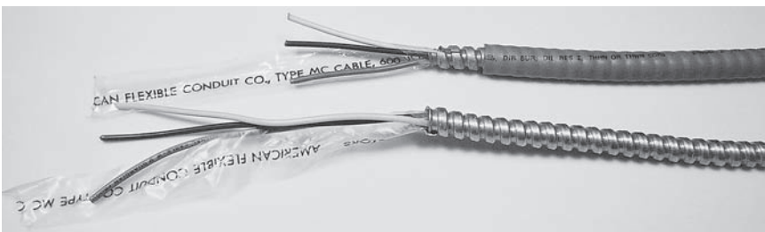
Fig. 11–33 Interlocking armor Type MC cable. The version at the top has an outer non-metallic jacket and is listed for direct burial.
