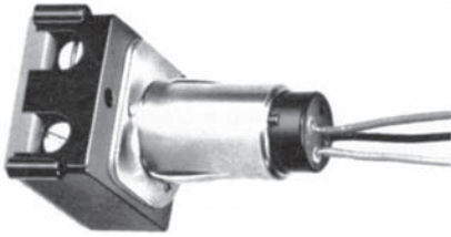
Fig. 19-4 The remote-control relay is an electrically operated switch. It is installed in either a master control panel or through a 1/2-in. knockout on the side of the outlet box on which the luminaire is mounted, depending on the application. ( General Electric Co. )
