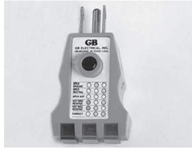
Fig. 18–30 This tester tells you whether 15- and 20-amp receptacles have been properly connected.
