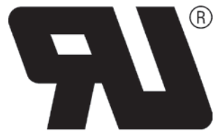
Fig. 1–5 Don't confuse this component recognition mark with a listing mark. (UL Inc.)
