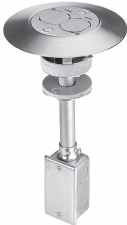
Fig. 31-1 A fire-rated poke-through assembly, designed for a 3-in. hole bored in a concrete floor. The wiring connections are all in the floor below, usually in a suspended ceiling cavity. ( Hubbell Electrical Products )
