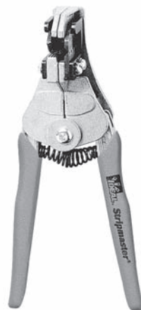
Fig. 8-1 A wire stripper saves much time in removing insulation. (Ideal Industries, Inc.)
