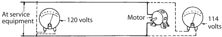
Fig. 2-8 This circuit illustrates voltage drop.
