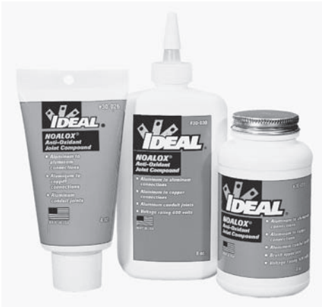
Fig. 8–26 One of several compounds available for treating aluminum connections. Apply it immediately after stripping the wire because raw aluminum develops an oxide skin almost immediately after exposure to air. (Ideal Industries, Inc.)
