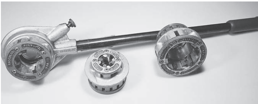
Fig. 11-5 This threader can be used for all conduit sizes 2 in. and smaller. Larger sizes require special geared threaders.
