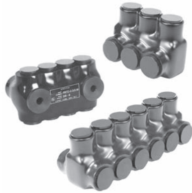
Fig. 8-14 These connectors are listed for a wide variety of finely stranded conductors, including Classes H, I, K, M, and DLO for diesel locomotive use. The internal bearing screw includes a pivoting, non-turning pressure plate that does not cut strands as it tightens. (Courtesy, Illsco .)
