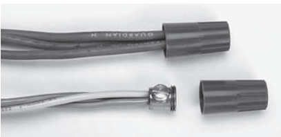
Fig. 8-15 Two types of solderless connectors for smaller wires, often called by the trade name "Wire Nut." The version with the setscrew maintains the integrity of the electrical connection even with the insulating cap removed. This makes it a good choice if the connection will be tested with diagnostic equipment while energized, such as with some motor connections.
