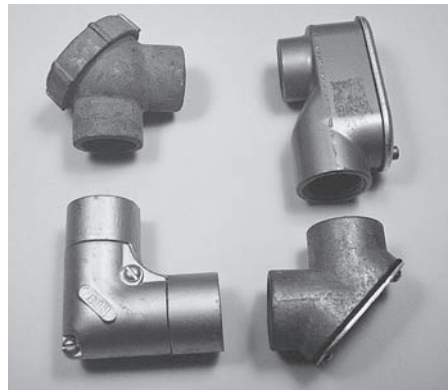
Fig. 27-3 "Short radius" conduit bodies only enable raceway installation and do not function as boxes. Due to restricted size, they cannot be used for 4 AWG or larger conductors.
