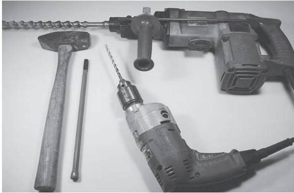
Fig. 21–20 To drill an occasional hole in masonry, use a star drill or a masonry chisel and a hammer, as at left. This method will put a hole through a wall for a conduit, but isn't precise enough to seat most anchors. Use a carbide-tipped drill bit with an electric drill, especially in the smaller sizes (center). Use a rotary hammer for larger holes. The one shown (upper right) compresses air behind the chuck in the process of rotation, delivering explosive impacts with each revolution that allow for rapid progress.
