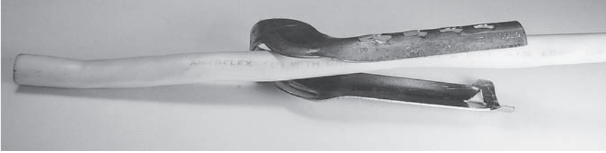
Fig. 11-27 This cable ripper saves much time in installing nonmetallic-sheathed cable.
