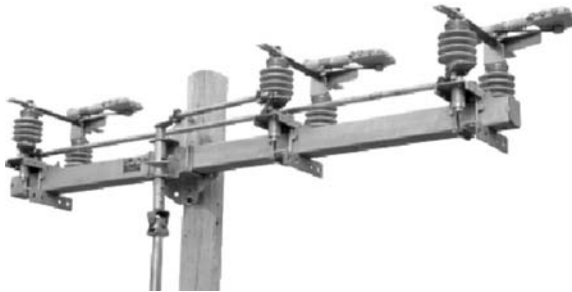
FIGURE 4.19 Typical side break switch disconnector showing operation rod and arc breaking chambers (Hubbell Power System Inc. Type AR, 15 kV 900 A continuous/interruption rating).
