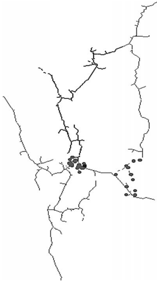
FIGURE 9.1 Geographical network diagram of the example long rural feeder used in case study 1.
