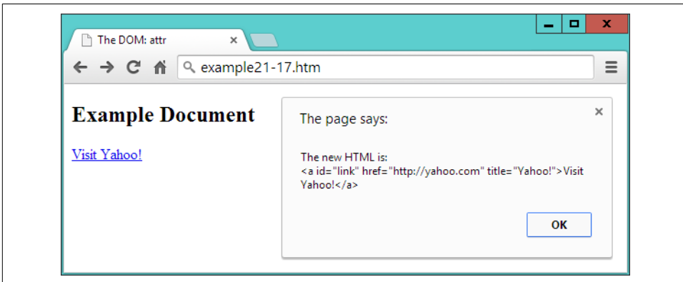
Figure 21-15. The link has now been completely modified
