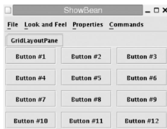
Figure 11-4. Components laid out with a GridLayout
