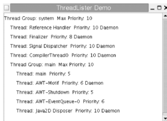
Figure 4-1. The threads and thread groups of a Swing application
