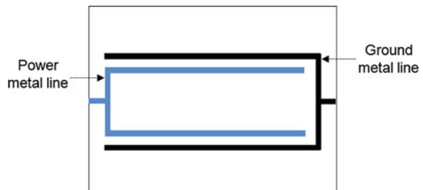
Fig. 7.9 Finger type based on-chip P/G metal lines
