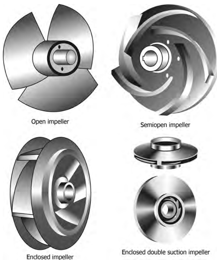
FIGURE 5.5 Open, semiopen, and enclosed impellers.
