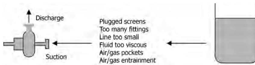
FIGURE 5.13 Pump suction side problems.
