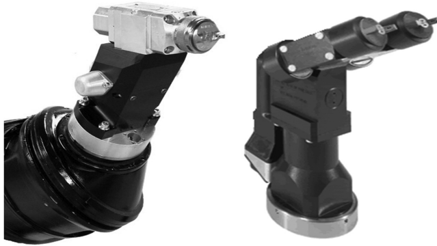
Figure 4.21 Dual and single-head spray applicators
