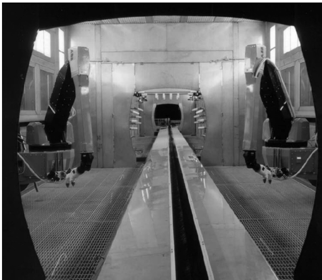
Figure 4.18 An automotive paint spray booth
