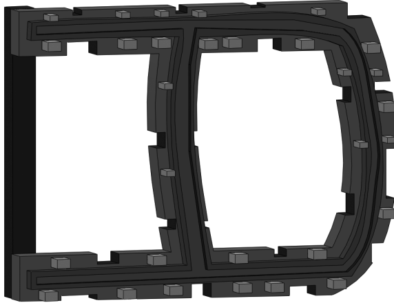
Figure 2.58 A hard fixture used for dimensional approval. Reproduced by permission of American Iron and Steel Institute and Auto/Steel Partnership © 2010
