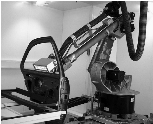
Figure 4.14 The UV curing robotic implementation
