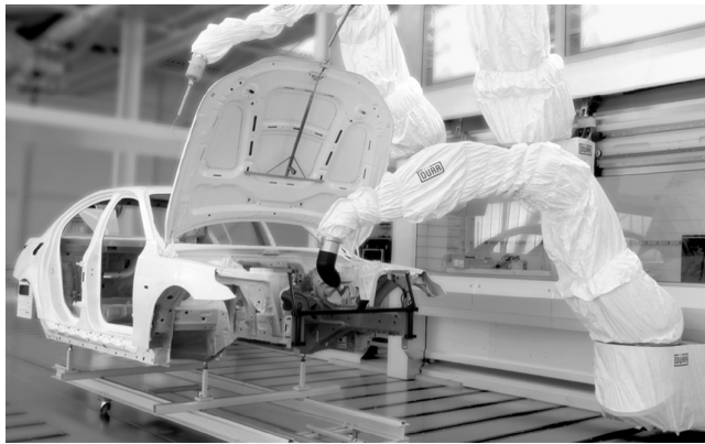
Figure 4.35 The different types of painting robots used in spray booths
