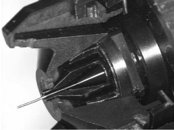
Figure 4.24 Internal charging of the paint
