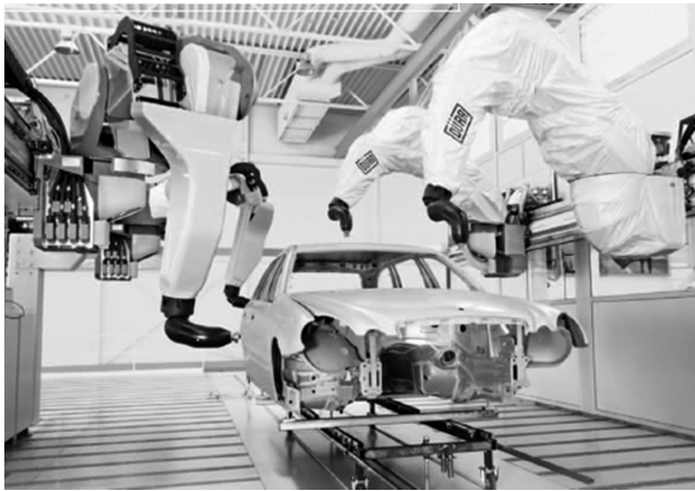
Figure 6.22 Overhanging robots. Reproduced by permission of Duerr Systems, Inc © 2010
