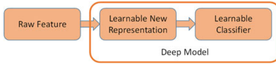
Fig. 9.1 Deep model jointly learns feature representation and classifier
