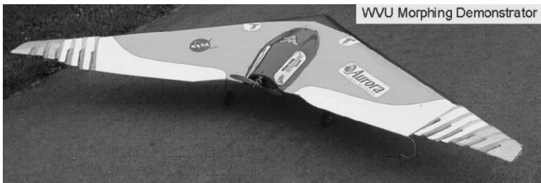
3.10 WVU swept-wing morphing demonstrator. (Source: Guiler et al. , 2008.)
