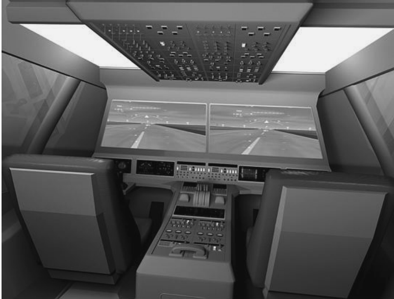
8.19 Synthetic vision system. (Source: NASA EL-1998-00169.)
