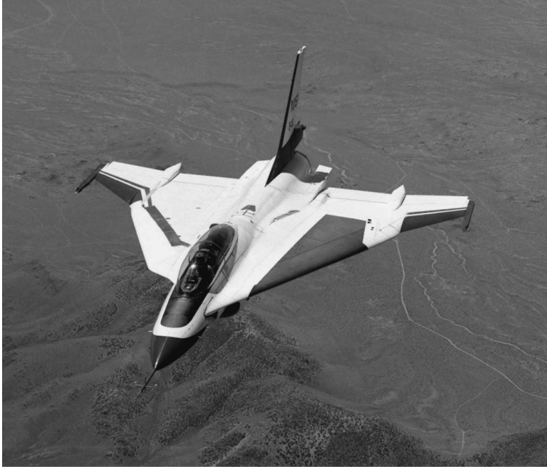
8.16 F-16XL with SLFC 'glove'. (Source: NASA EC96-43548-8.)
