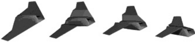
3.5 Lockheed Martin morphing adaptive structures (MAS) demonstrator. (Source: Ivanco et al. , 2007.)
