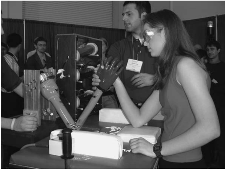
2.14 The robotic arm driven by artificial muscles, made by Virginia Tech students, is being prepared for the 2005 match against the human opponent.
