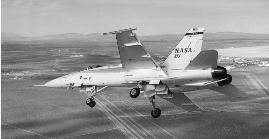
3.3 NASA-Boeing F/A-18A incorporating the active aeroelastic wing (AAW). (Source: Curry, 2005.)
