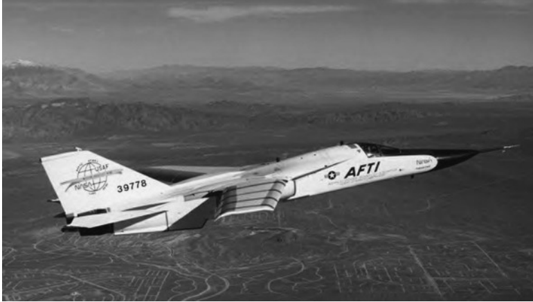
3.2 NASA-Boeing F-111 incorporating the mission adaptive wing (MAW). (Source: Curry, 2004.)
