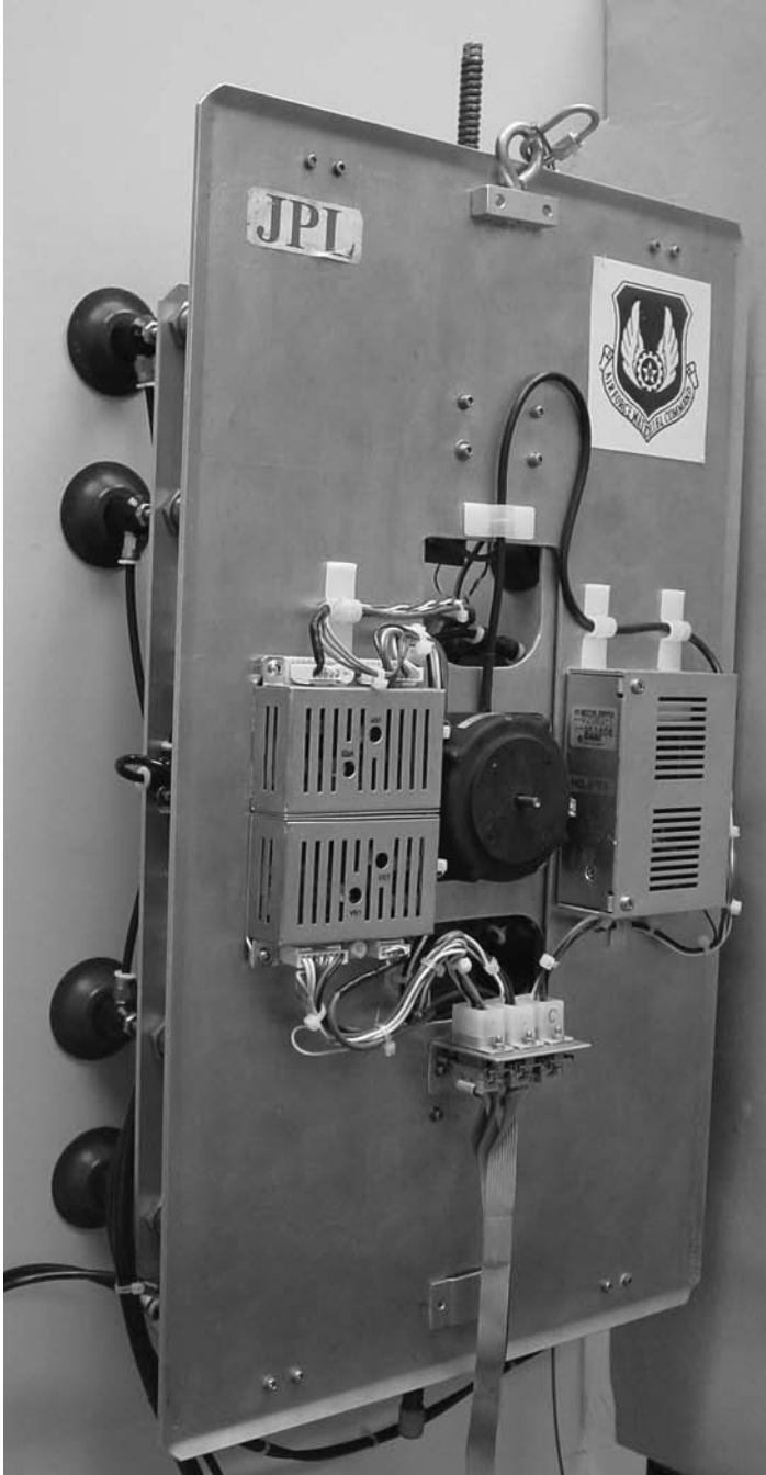
2.15 MACS crawling on a wall using suction cups on two simulated legs.
