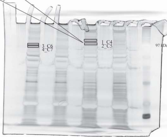
Fig. 12. Example of LC-MS/MS identification of gel-separated proteins in a gel contaminated with a high background of IgG and keratin. (Collaborator: Y. Xiong.)
