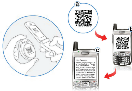
Fig. 9. A procedure for temperature data collection using a wearable sensor and a mobile phone. (a) A QR code image. (b) A QR code captured by a camera built into a mobile phone. (c) Original data recovered from the image captured by a mobile phone (QOL Co. Ltd., 2008).
