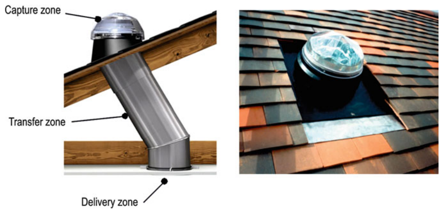
Fig. 13.12 Example of a light pipe for residential application (courtesy of Solatube Co.)
