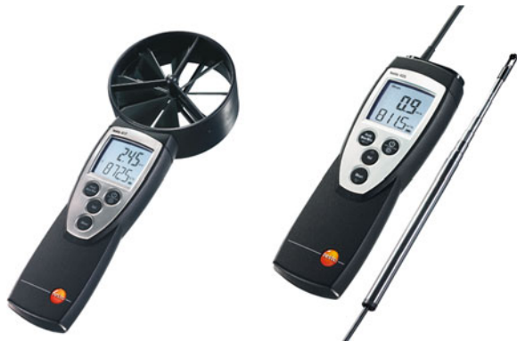
Fig. 5.4 Example of portable anemometers: on the left vane type on the right hot-wire type (courtesy of Testo AG)
