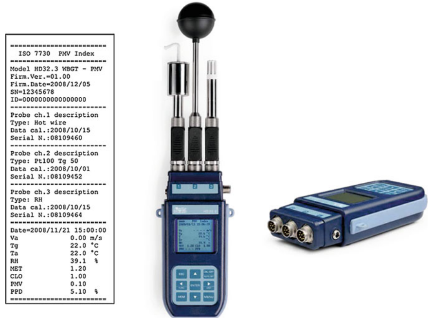
Fig. 5.7 Example of microclimate analyser (courtesy of Delta Ohm— www.deltaohm.com )
