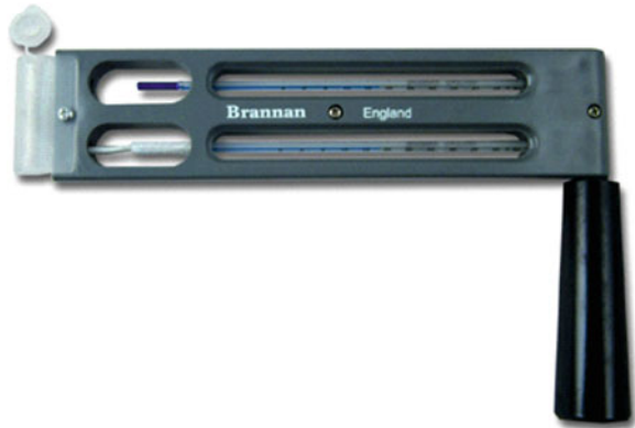
Fig. 5.5 Example of sling psychrometer for measuring relative humidity (courtesy of Brannan Co.
