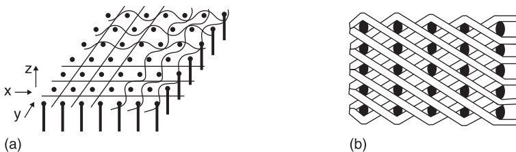
3.9 (a) 3D weave, the simplest structure; (b) multilayer 3D weave with x/y warp direction and z weft direction.
