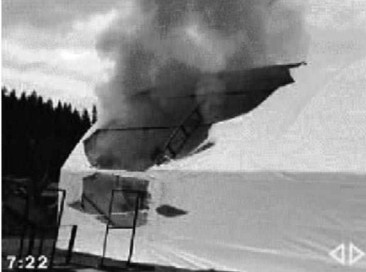
12.49 Fire behaviour during tests of PVC-coated polyester material, flames perforate the membrane, exacuating smoke and heat (FERRARI tests).
