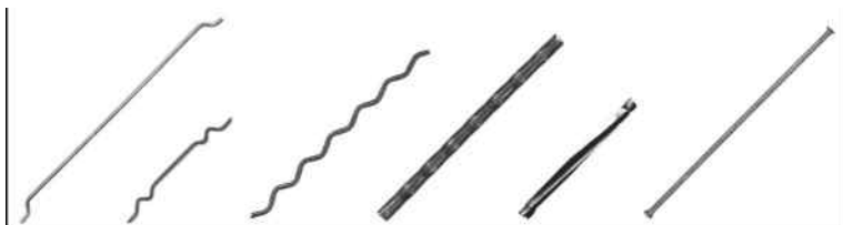
1.7 Different types of steel fibres used for concrete reinforcement.
