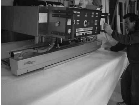
12.53 High-frequency electrode for welding.
