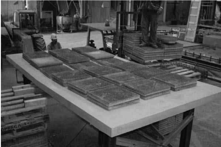
4.35 Final view of the panel, loaded with 33 concrete plates.
