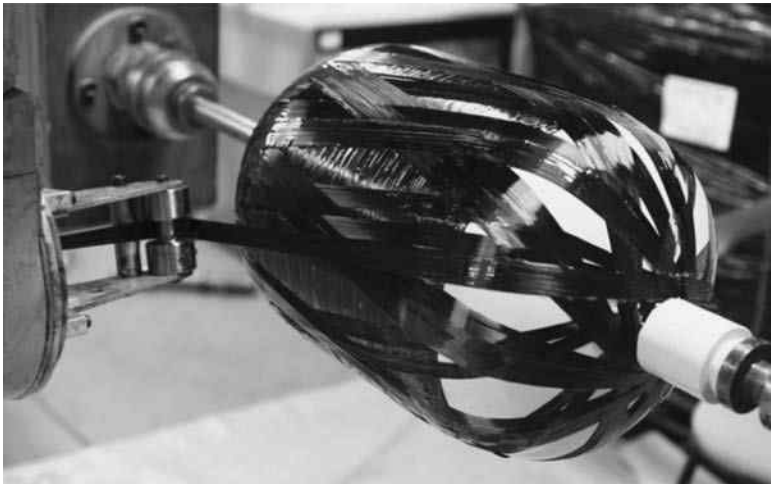
7.6 Filament winding process.
