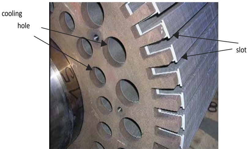
Figure 4.5. Detail view of a squirrel rotor being built. Note the cooling holes (photo source: Converteam)
