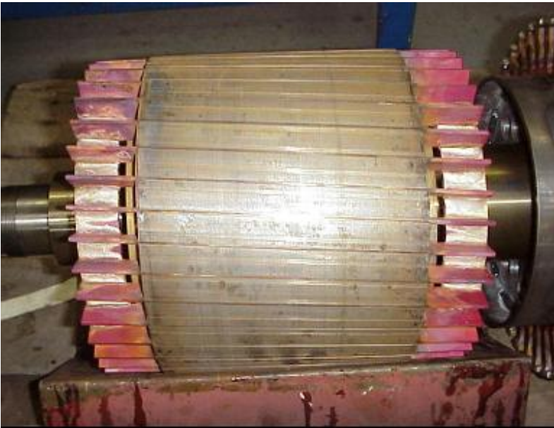
Figure 4.3. Squirrel rotor of induction machine, 6 kVA, 440 V, 60 Hz, 1 200 rpm. Note the skew of the slots (ECA EN document)
