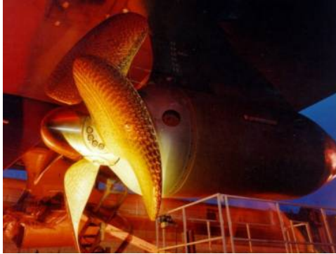
Figure 3.34. Motor in a pod fixed under the hull of a ship (photo source: Converteam)
