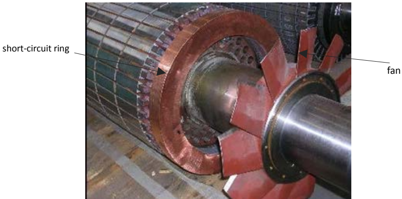
Figure 4.6. Squirrel rotor. The short-circuit ring connecting the bars to one another is visible as well as the fan on the shaft (photo source: Converteam)
