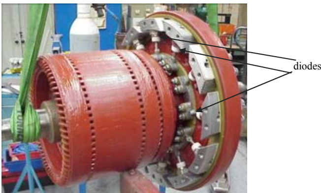
Figure 3.27. Rotor of a “rotating diode” exciter, 155 kVA, 74 V, 3,000 rpm. On the right hand side of the photograph the semi-conductor components are distinctly visible enabling the armature currents of the inverted AC generator (ECA EN document) to be rectified
