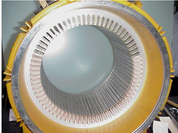
Figure 4.1. Induction machine stator before winding, 45 kW, 440 V, 590 rpm (ECA EN document)
