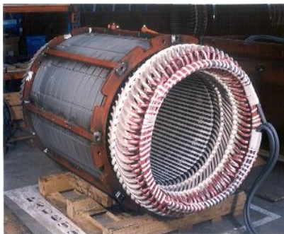
Figure 3.1. Synchronous machine stator (photo source: Convertteam)
