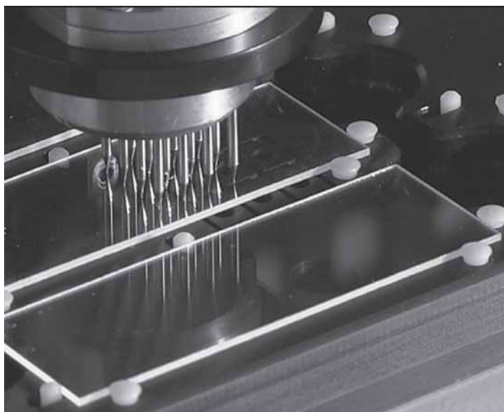
Fig. 7. Contact printing using solid pins provides a rapid, convenient method for fabrication of protein microarrays on many different surfaces.
