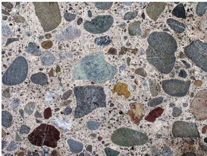
Fig. 1.7 Concrete —A concrete in its hardened state consists of hydrated cement paste, Fine aggregates (usually, sand) and coarse aggregates (crushed stone particles). It formed when the cement hydrates in the presence of water and leads to the formation of different products of hydration that, later on, fill in the empty spaces left between different constituents of the concrete and finally, giving it a capacity to support the load
