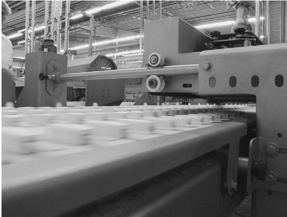
Figure 16.6 Stickline for ice-cream products (Gram)
