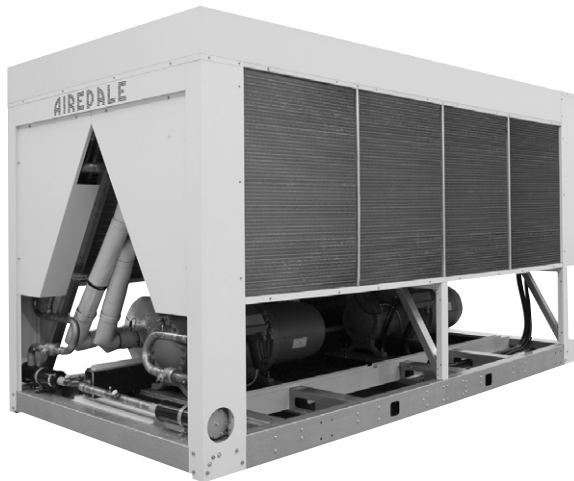
Figure 13.7 Air-cooled water chiller, nominal 600 kW capacity with two R134a refrigerant circuits, single shell and tube evaporator, and capacity controlled semi-hermetic screw compressors (Airedale)
