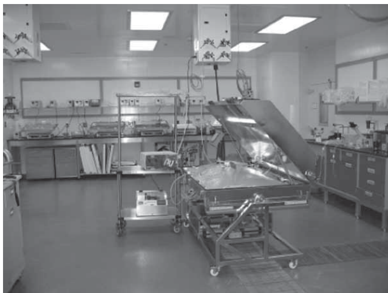
Fig. 1. Photograph of Wave System200EH with inflated Cellbag200 set up in GSK RTP fermentation facility. In the background, System20s and System50s can be seen.
