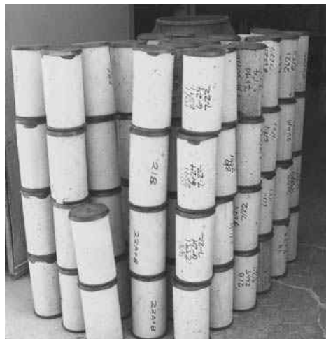
Standard capped cylinders ready for testing.
