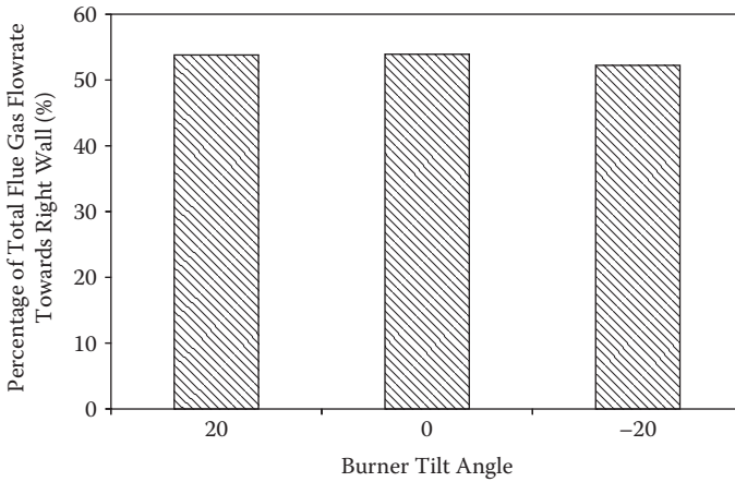
FIGURE 5.11 Influence of burner tilt on mass flow distribution in the crossover pass (front RH).
