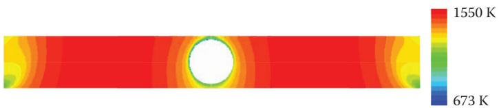
COLOR FIGURE 4.14 Simulated temperature distribution across a tube of a typical platen superheater.
