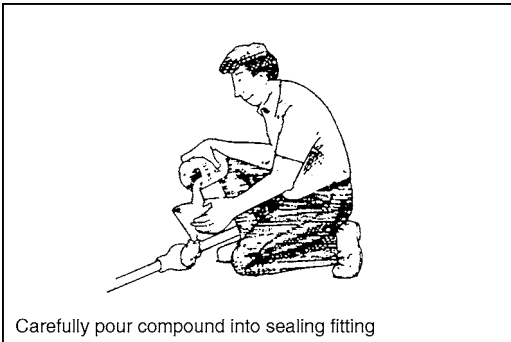
FIGURE 9-4. Carefully pour compound into sealing fitting.
