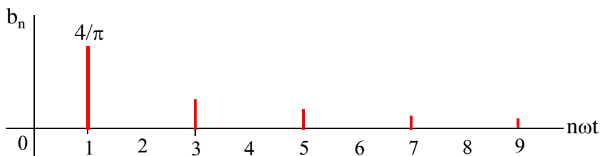
Figure 7.34. Line spectrum for square waveform in Subsection 7.4.1
