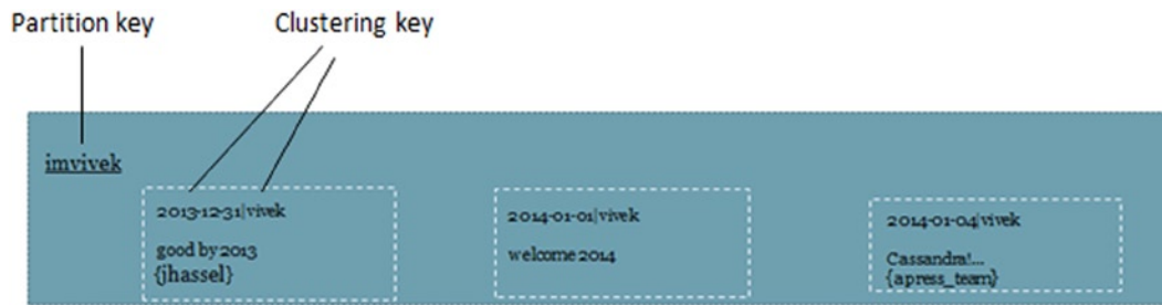
Figure 3-7. Composite column having invivek as the partition key and remaining as the cluster key
